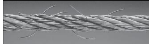
Cable with Broken Wires
