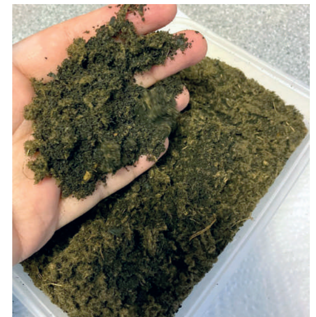
After 24 hours, the biowaste had indeed been transformed into a peat-like product. In the process, around 42% of the weight was lost in the form of water. At an electrical efficiency of 14%, however, that water loss came at quite a price. Treating one tonne of biowaste in the machine costs more than € 700.
