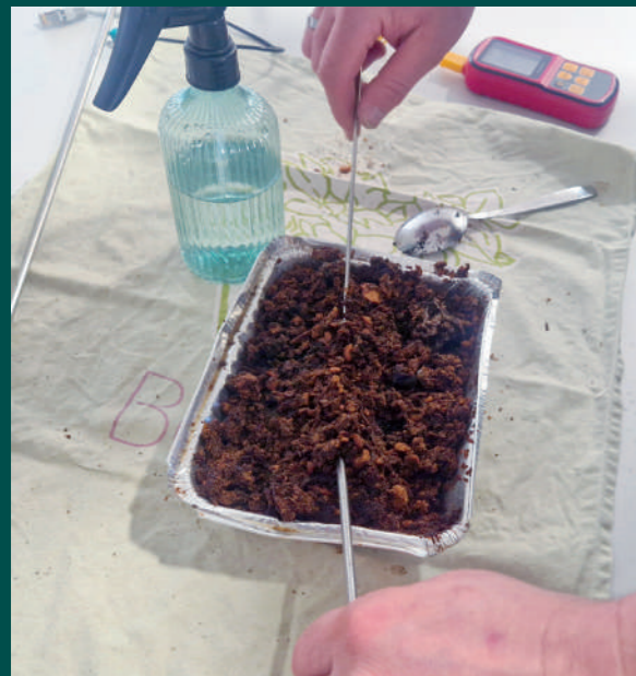
Unfortunately, after 24 hours of composting, the product was not stable and began to heat up again after being remoistened.
