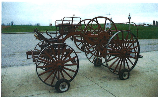
There was a lot of work in getting the wheels on this P.J. Cooney hose cart freed from the axle as the hub was welded to the axle and the steel pipe was welded to the hub. The hubs were saved, the wheels were rebuilt and new brass hub caps made.
