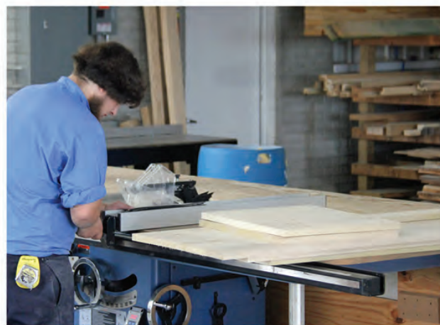
An employee in the Weaver Wagons manufacturing facility as he adjusts a saw to cut a side board.
