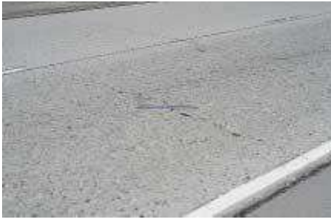
Figure 4.95: JCP High Severity Transverse Cracking
