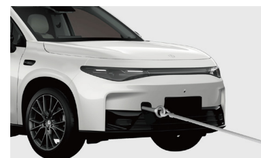
Towing hook installation location
