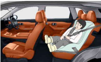
Group II child safety seat: Suitable for children weighing 15kg to 25kg.
