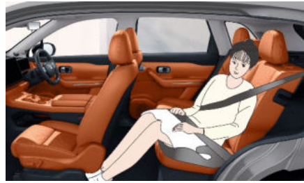
Group III child safety seat: Suitable for children weighing 22kg to 36kg.
