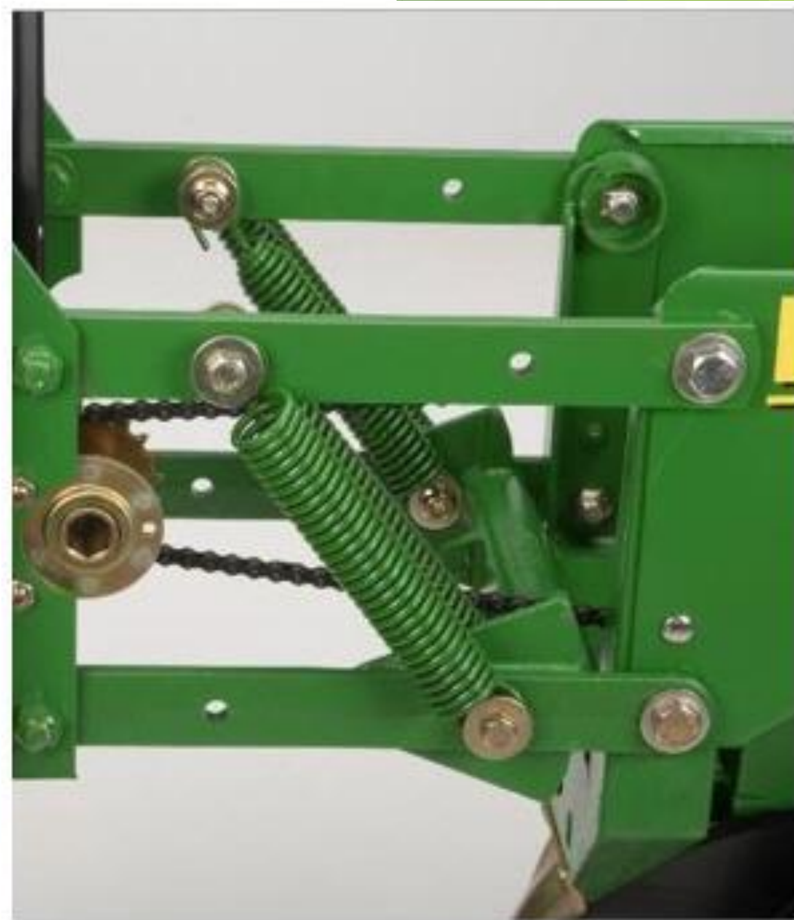
Upforce springs on a standard row-unit
