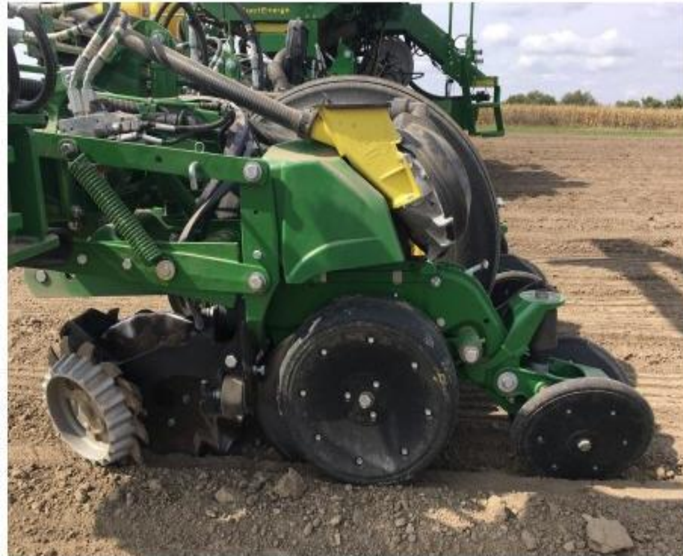
One set of upforce springs on long parallel arms with IRHD
