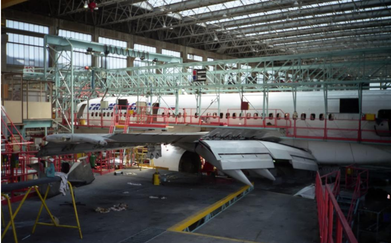
Figure 1: A Boeing 757 airliner undergoing a heavy maintenance “C-check” at a maintenance hangar (British Airways Engineering base at Heathrow). Such airframe heavy maintenance visits involve extensive structural inspection, overhaul of systems, and necessary repairs/modifications. Large commercial jets typically require heavy checks every 5–10 years of service.
