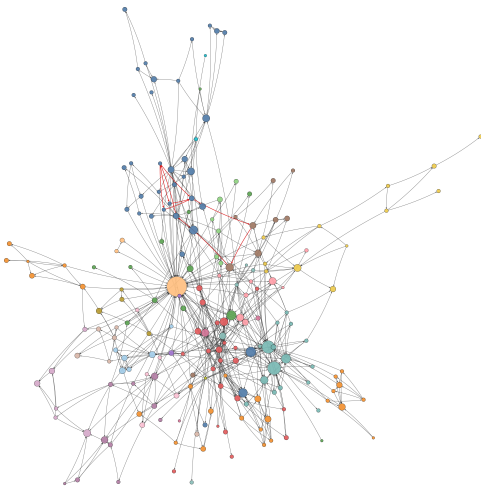
Figure 1. A dependency graph of the OpenHands SDK [10]. Nodes correspond to files in the openhands.sdk module, and edges to imports (oriented from importers to importees). Node size is scaled with the number of incoming edges. The red edges indicate cycles in the import structure.
