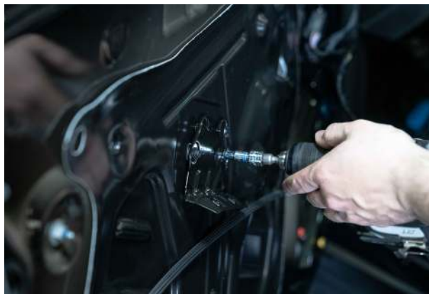
▲ Figure 32. Removing the door handle bracket.
