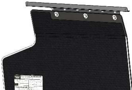
▲ Figure 62. Rendering of the armor and Upper Mounting Bracket showing relative location and placement.
