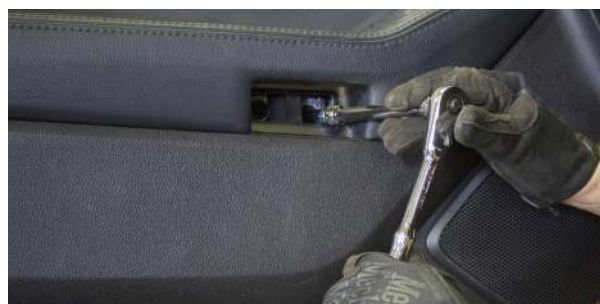
▲ Figure 26. Removing the armrest pocket bolts.
