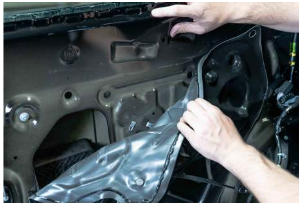
▲ Figure 33. Removing the weather seal.
