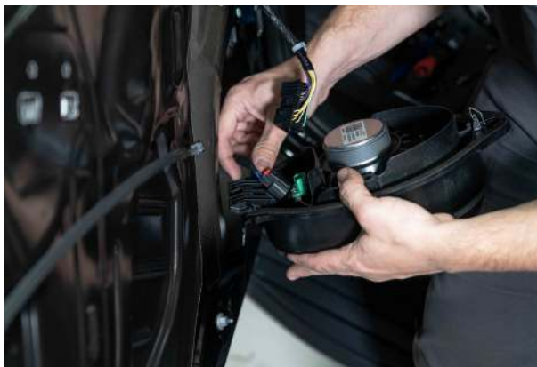
▲ Figure 31. Disconnecting the speaker harness.
