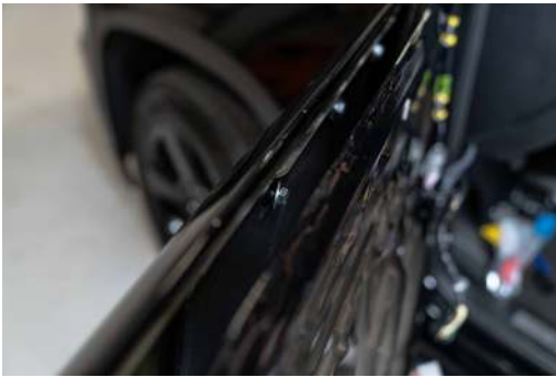
▲ Figure 61. Loosely installed upper mounting bracket..
