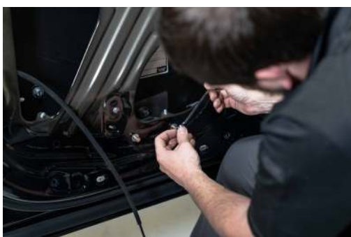
▲ Figure 73. Installing the lower mounting bracket.
