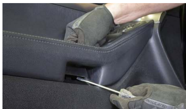
▲ Figure 25. Removing the armrest pocket trim cover.
