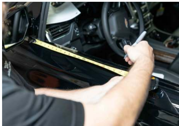
▲ Figure 45. Marking Bracket locations.
