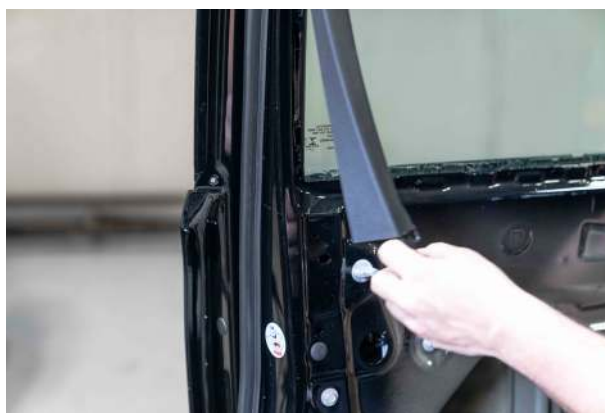
▲ Figure 35. Removing the window trim.
