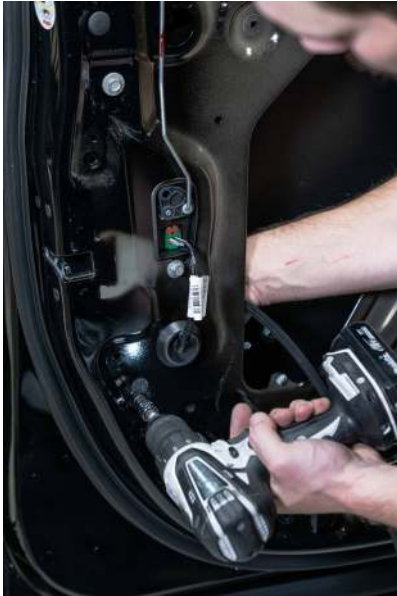
▲ Figure 76. Loosening the rear window track.
