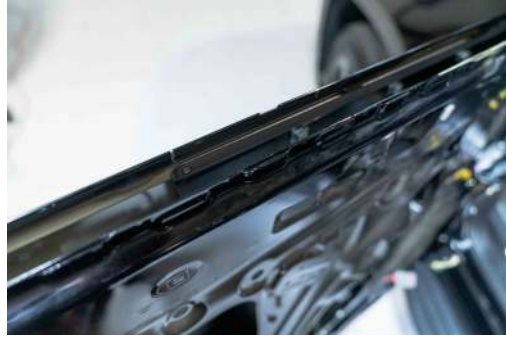
▲ Figure 66. Support Bracket aligned and installed.
