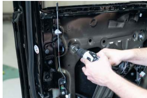
▲ Figure 72. Tightening the regulator mounting bolt.
