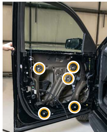
▲ Figure 41. Location of the 5 window regulator fasteners.
