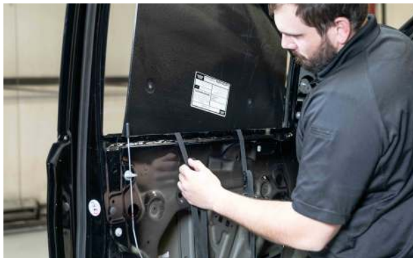
▲ Figure 55. Placing the armor into the door.
