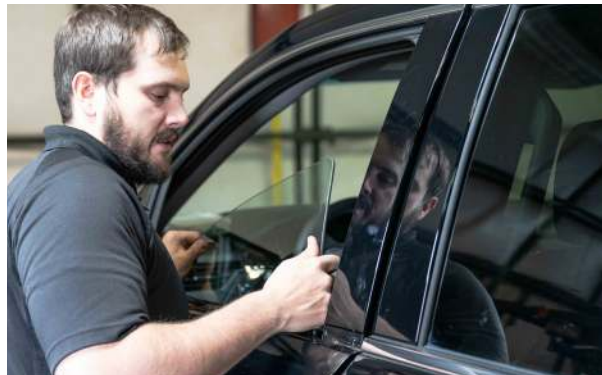
▲ Figure 39. Removing the window glass.
