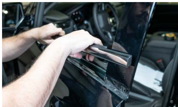
▲ Figure 24. Removing the outer window weatherstrip.
