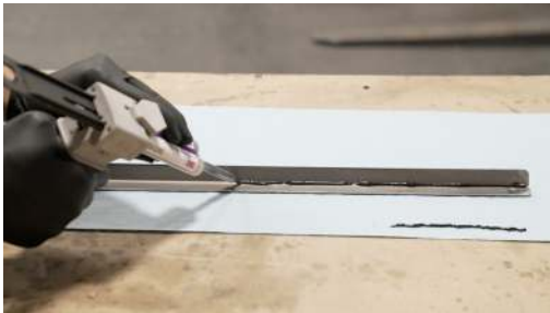
▲ Figure 64. Applying panel bond to support bracket.
