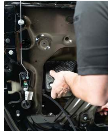
▲ Figure 48. Prying out the foam block.
