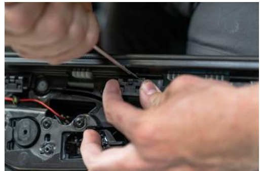
▲ Figure 78. Removing the metal clip from the interior panel.
