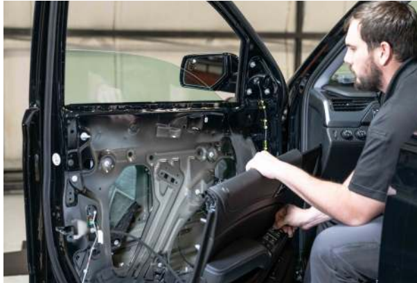
▲ Figure 38. Moving the window down.
