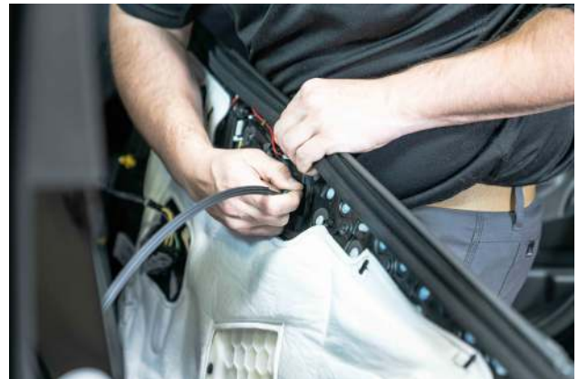
▲ Figure 30. Removing the door latch cable.
