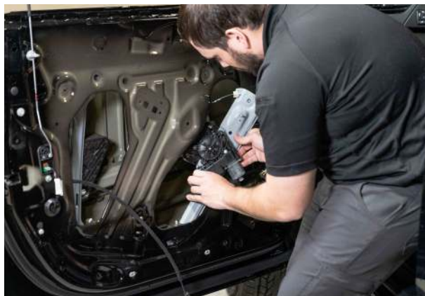
▲ Figure 42. Removing the window regulator.
