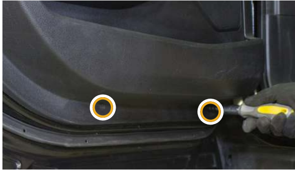
▲ Figure 27. Removing the door panel bolts.
