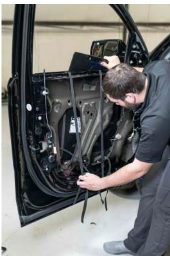
▲ Figure 56. Using the cradle created by the installation straps to lower the armor into the door.
