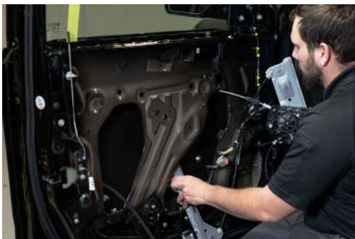
▲ Figure 71. Inserting the rear section of the window regulator.
