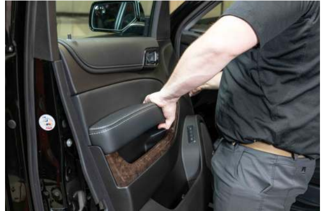
▲ Figure 29. Tilting the door panel away from the door skin.
