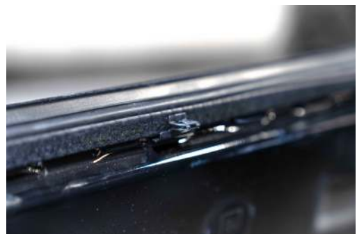
▲ Figure 79. Metal clip reinstalled to the door with the weatherstrip over the top.
