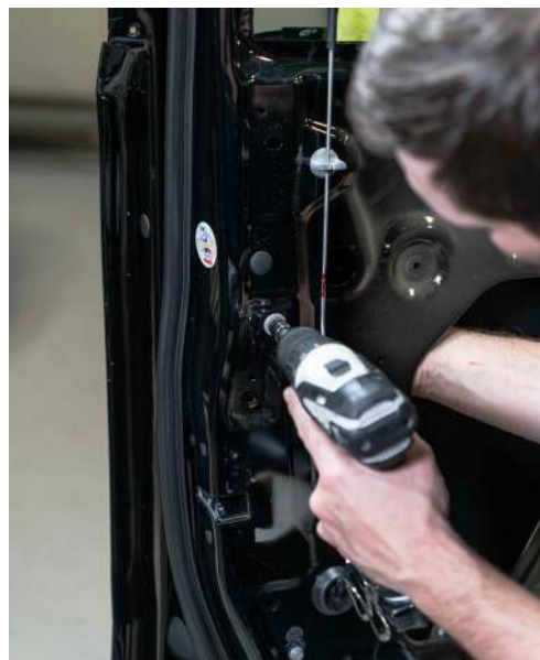
▲ Figure 75. Remove the upper window track bolt.
