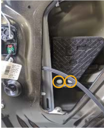
▲ Figure 47. Location of the two foam mounting clips.
