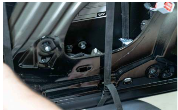
▲ Figure 57. The front, top of the crash bar bracket loosely installed.
