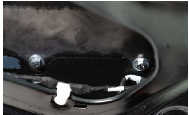
▲ Figure 77. Showing bolts that loosely install the crash bar
