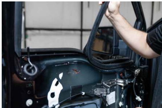
▲ Figure 33. Removing the inner weather stripping
