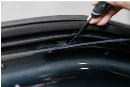
▲ Figure 30. Removing the outer window weatherstrip
