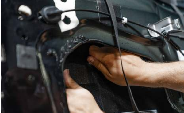
▲ Figure 78. Loosely attaching the mounting bracket
