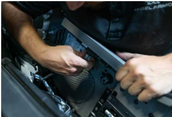
▲ Figure 27. Removing the door panel
