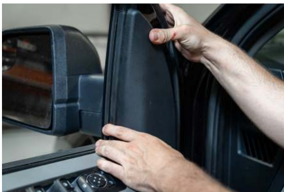
▲ Figure 19. Removing the trim panel
