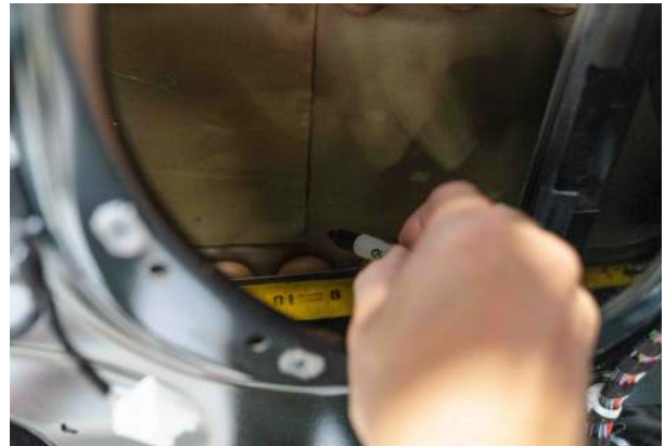
▲ Figure 71. Marking 9.25 inches toward the rear of the vehicle from the front of the crash bar
