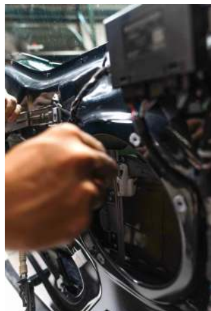
▲ Figure 36. Disconnecting the front clip
