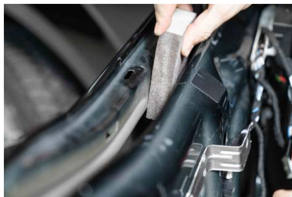
▲ Figure 57. Removing rust, primer and paint
