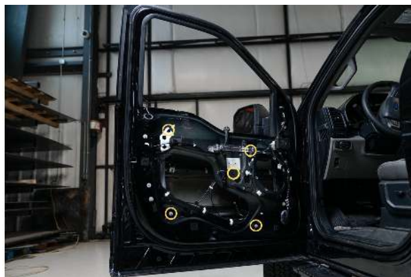
▲ Figure 39. Locating the hex nuts and bolt
