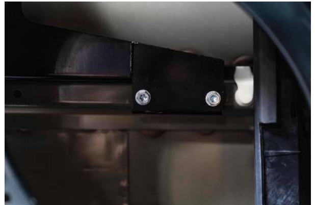
▲ Figure 68. Sheet metal screws mounted to crash bar
