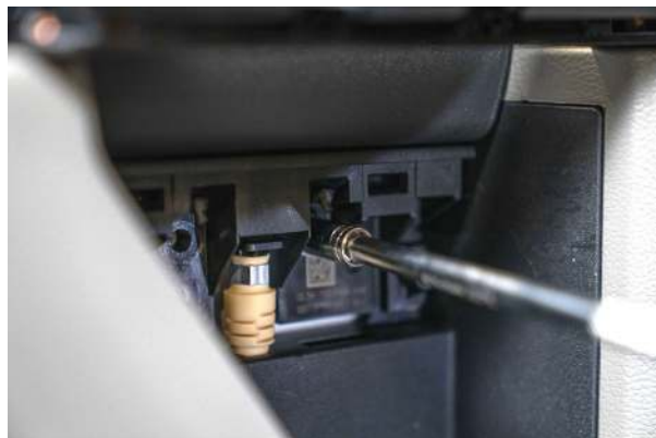
▲ Figure 24. Removing the interior door handle bolts
