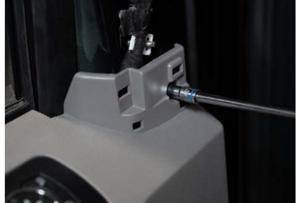
▲ Figure 20. Removing the screw behind the mirror trim panel
