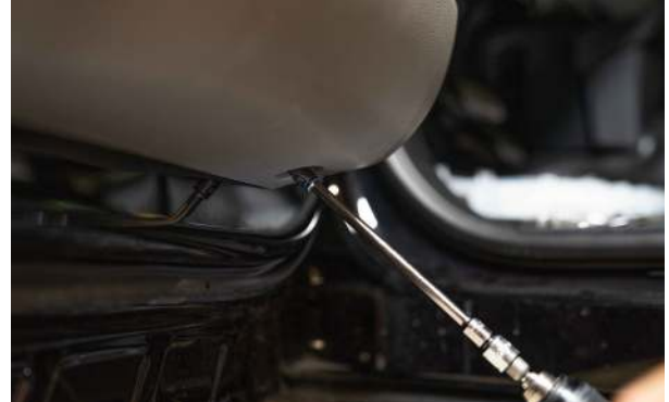
▲ Figure 25. Removing the lower panel bolts
