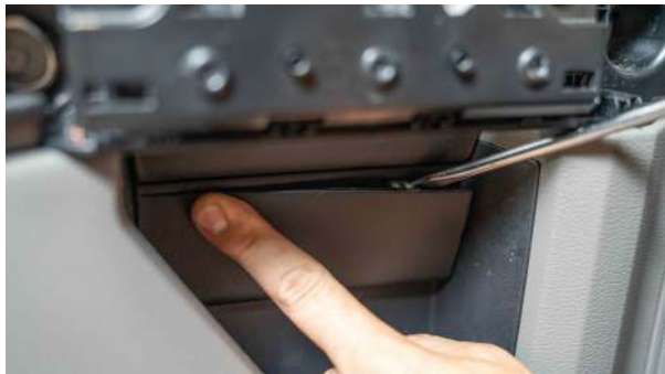
▲ Figure 23. Removing the trim panel below the latch
