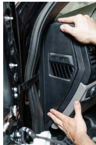
▲ Figure 54. Reinstalling the dash piece
