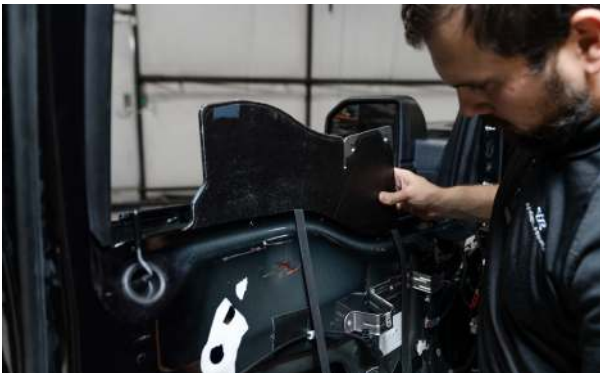
▲ Figure 76. Placing the armor into the door
