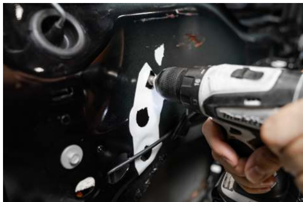
▲ Figure 41. Punching out the adhesive foam
