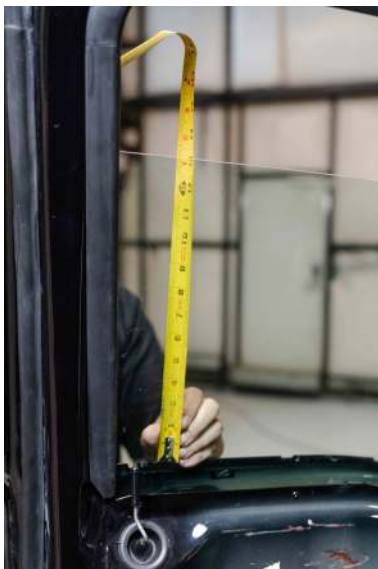
▲ Figure 32. Setting window height to 13 inches
