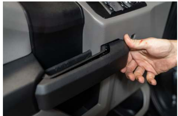
▲ Figure 22. Removing the handle panel
