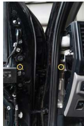
▲ Figure 47. Circular rivets in the door
