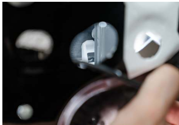
▲ Figure 34. Locating the window regulator clips
