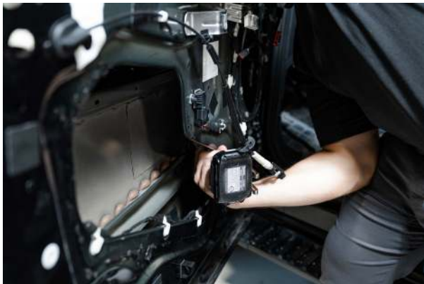
▲ Figure 70. Screwing in upper bracket
