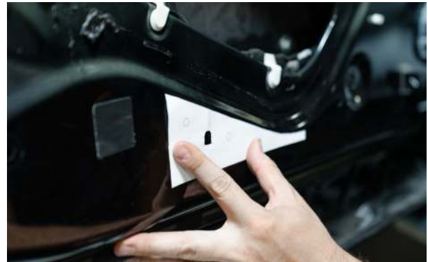
▲ Figure 80. Positioning the drill template
