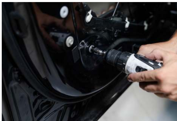
▲ Figure 42. Removing the window regulator mounting nuts
