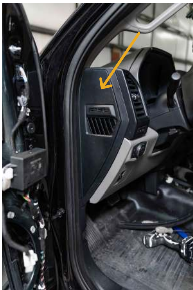
▲ Figure 45. Triangular trim piece to remove
