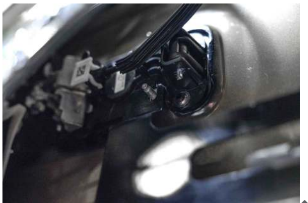
▲ Figure 63. Position of the rear portion of the upper bracket
