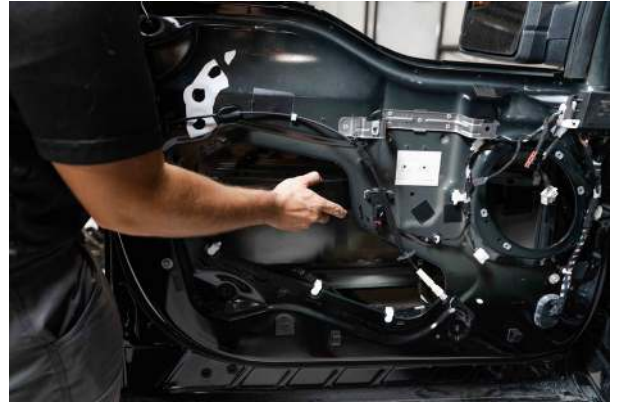
▲ Figure 67. Inserting the bracket into the door
