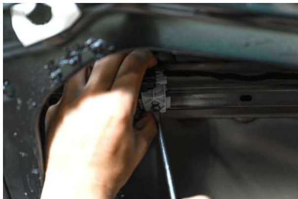
▲ Figure 55. Disconnecting wiring harness
