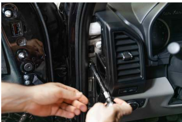
▲ Figure 51. Removing the dash frame
