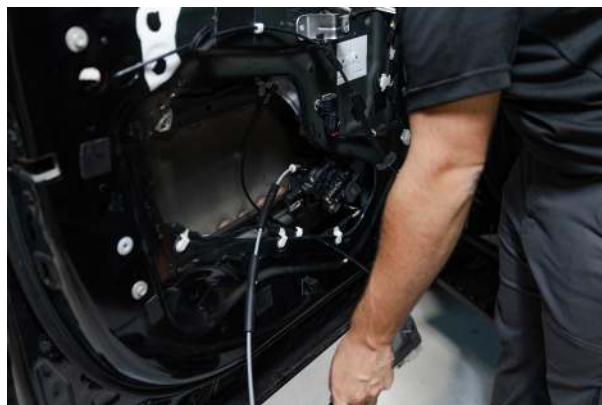
▲ Figure 44. Removing window regulator
