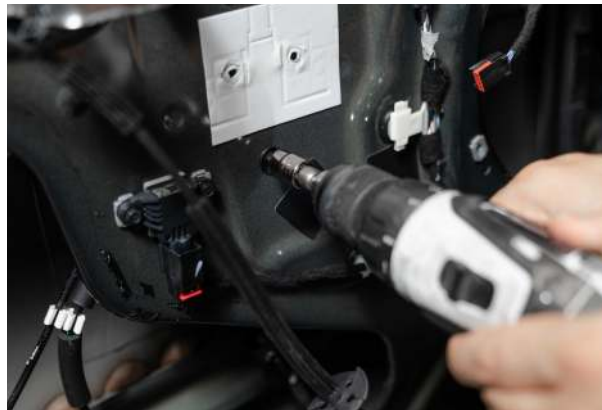
▲ Figure 43. Removing bolt from window regulator
