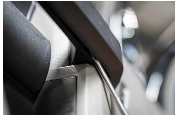
▲ Figure 21. Prying the trim panel loose
