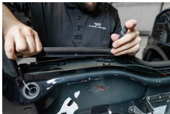
▲ Figure 31. Removing the outer window weatherstrip
