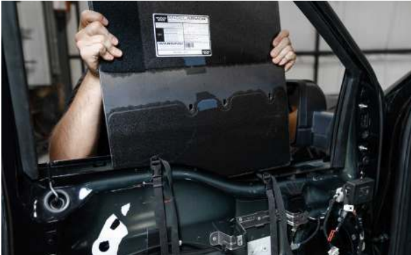
▲ Figure 75. Placing the armor into the door
