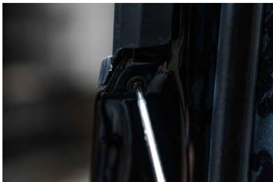
▲ Figure 29. Removing the back window weatherstrip screw
