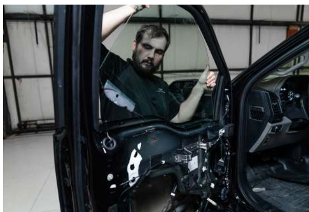
▲ Figure 37. Removing the window glass
