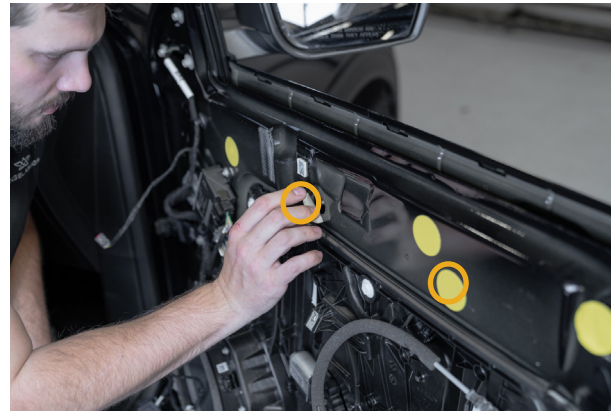
▲ Figure 37. Removing the adhesive patches
