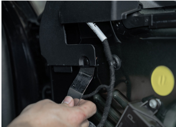
▲ Figure 43. Removing window trim from clips
