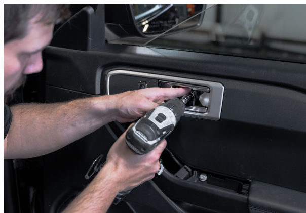
▲ Figure 24. Removing the interior door handle bolt
