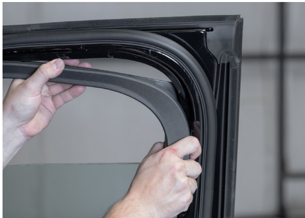
▲ Figure 44. Removing window trim
