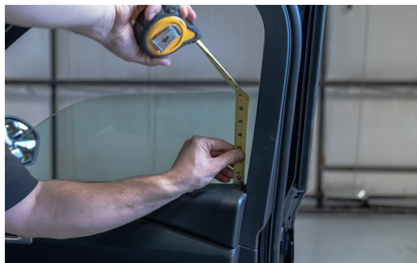
▲ Figure 32. Measuring the window height
