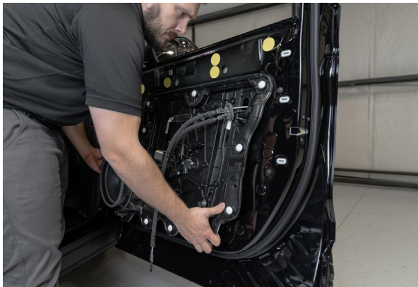
▲ Figure 39. Removing window regulator panel
