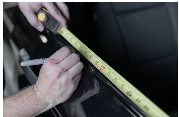
▲Figure 42. Measuring for the upper and supporting brackets
