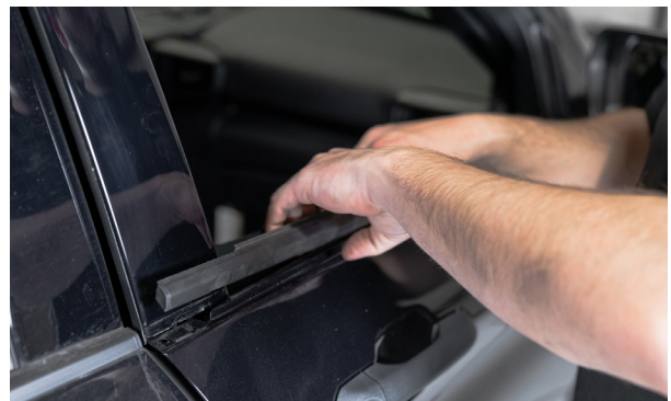
▲ Figure 22. Removing the outer window weatherstrip
