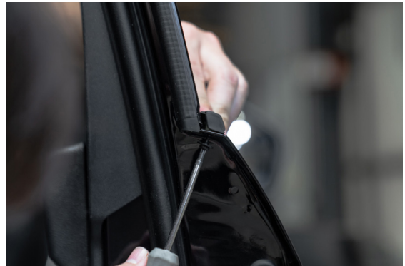
▲ Figure 21. Removing the back window weatherstrip screw
