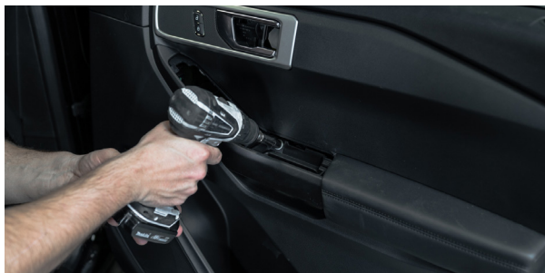
▲ Figure 26. Removing the armrest pocket bolts
