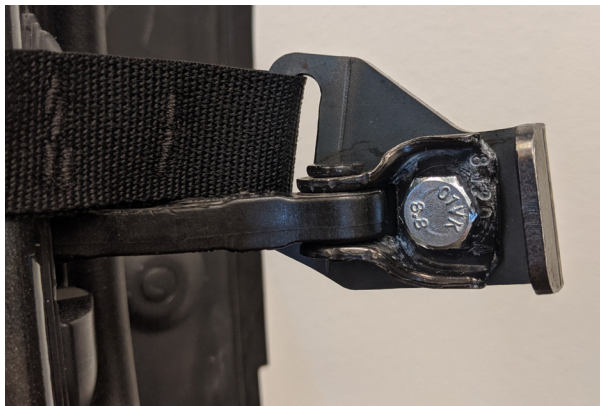
▲ Figure 47. Check strap orientation on A-pillar
