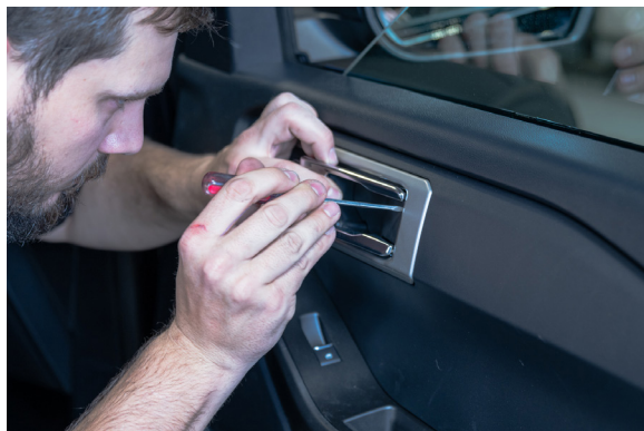
▲ Figure 23. Remove the interior door handle trim cover
