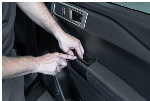
▲ Figure 25. Removing the interior door handle bolt
