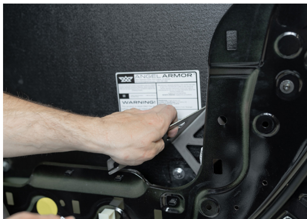
▲ Figure 56. Inserting Lower Mounting Bracket
