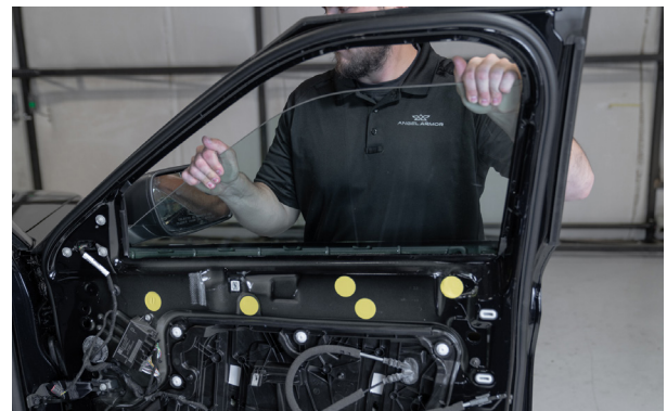
▲ Figure 34. Removing the window glass
