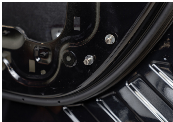
▲ Figure 57. Lower mounting bracket loosely installed
