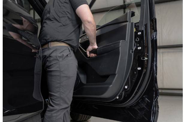
▲ Figure 29. Removing the door panel
