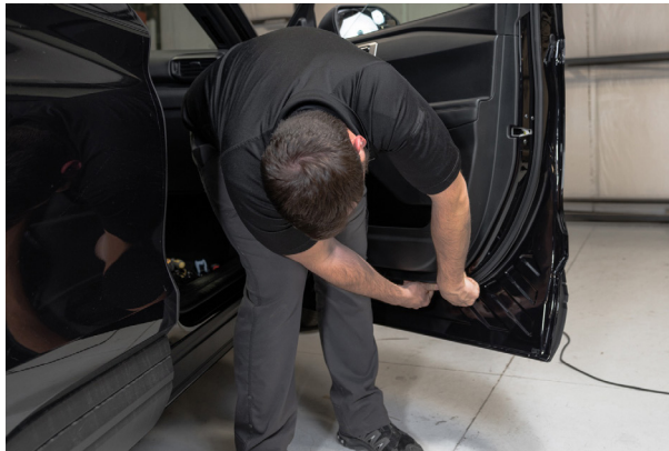
▲ Figure 28. Prying the door panel away from the door skin
