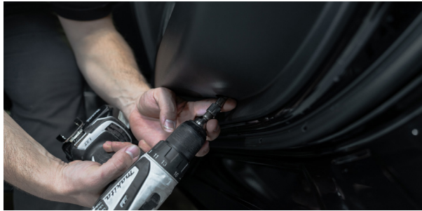
▲ Figure 27. Removing the lower panel bolts
