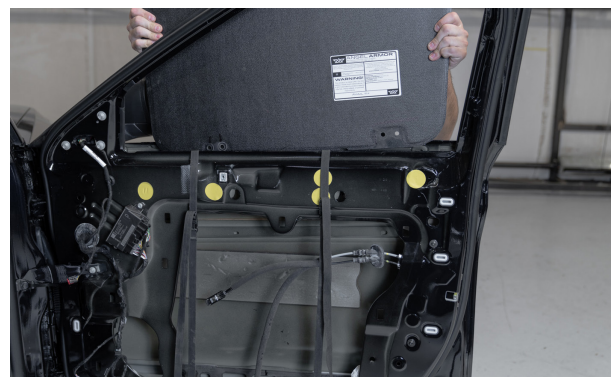
▲ Figure 53. Placing the armor into the door
