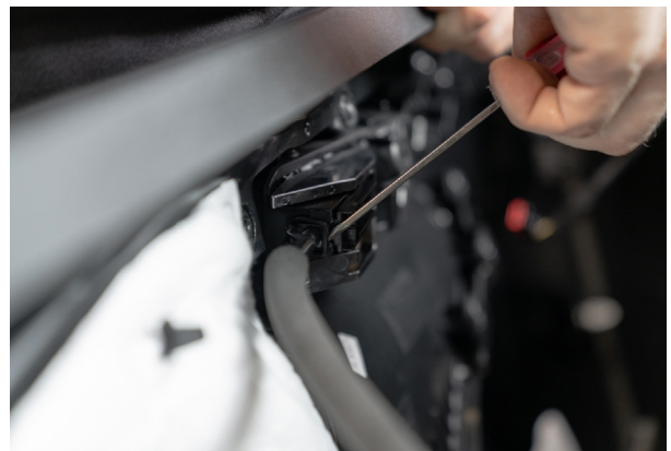
▲ Figure 30. Unclipping the door latches
