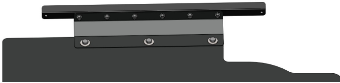
▲ Figure 63. Sheet metal screw locations
