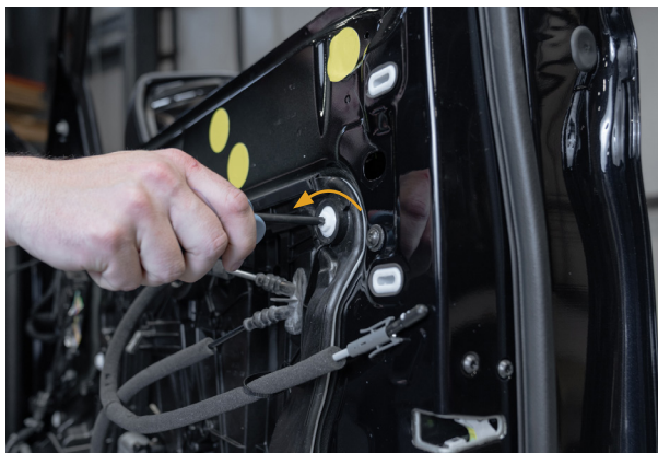
▲ Figure 36. Rotating Torx Clips
