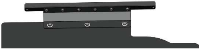
▲ Figure 63. Sheet metal screw locations
