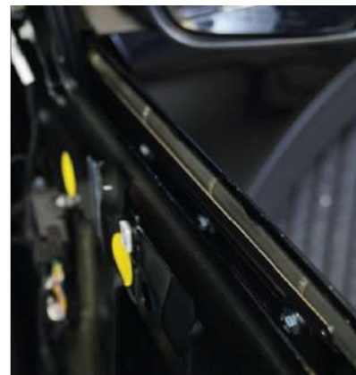
▲ Figure 59. The support bracket dry fitted into door
