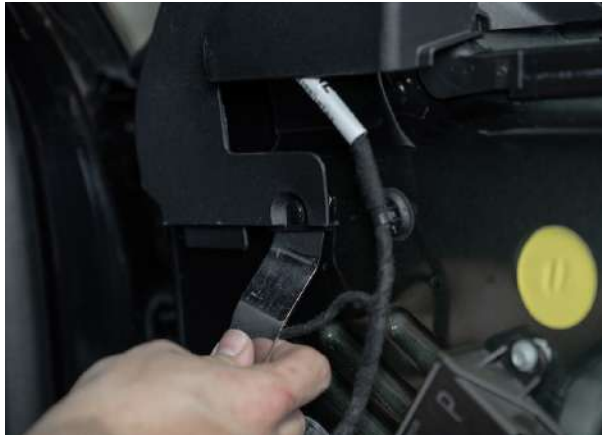
▲ Figure 43. Removing window trim from clips
