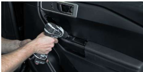
▲ Figure 26. Removing the armrest pocket bolts
