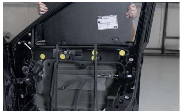
▲ Figure 53. Placing the armor into the door
