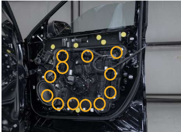
▲ Figure 35. Locating the mounting clips
