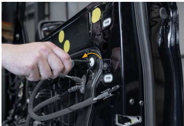
▲ Figure 36. Rotating Torx Clips
