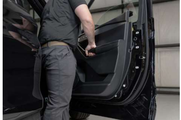
▲ Figure 29. Removing the door panel
