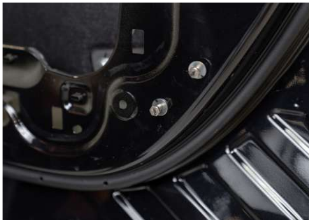
▲ Figure 57. Lower mounting bracket loosely installed
