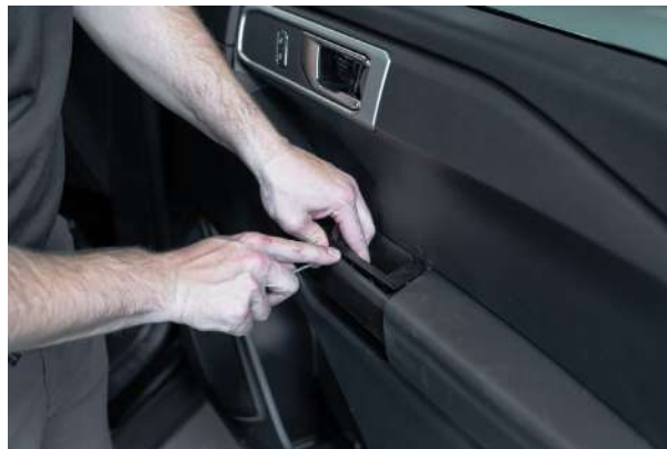
▲ Figure 25. Removing the interior door handle bolt
