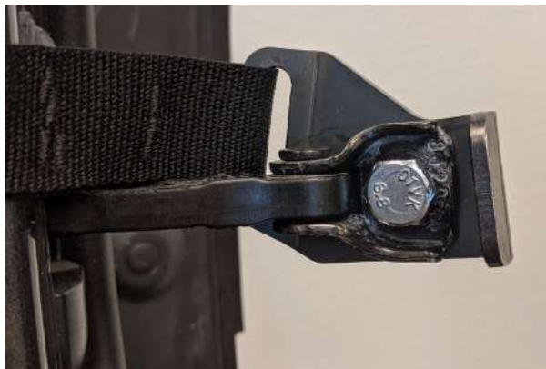
▲ Figure 47. Check strap orientation on A-pillar
