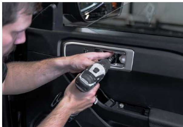
▲ Figure 24. Removing the interior door handle bolt
