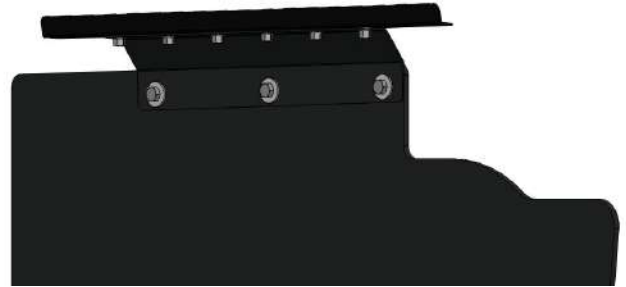
▲ Figure 58. Rendering of the armor and upper mounting bracket showing relative location and placement
