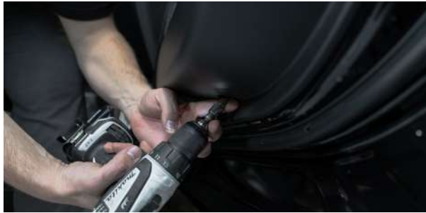
▲ Figure 27. Removing the lower panel bolts
