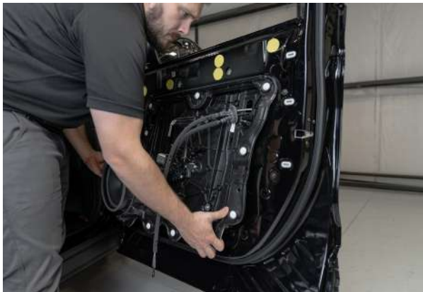
▲ Figure 39. Removing window regulator panel
