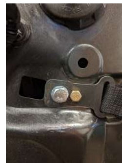
▲ Figure 46. Check strap mounting on the door
