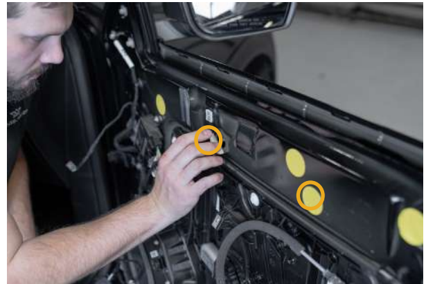
▲ Figure 37. Removing the adhesive patches
