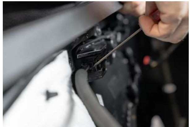
▲ Figure 30. Unclipping the door latches
