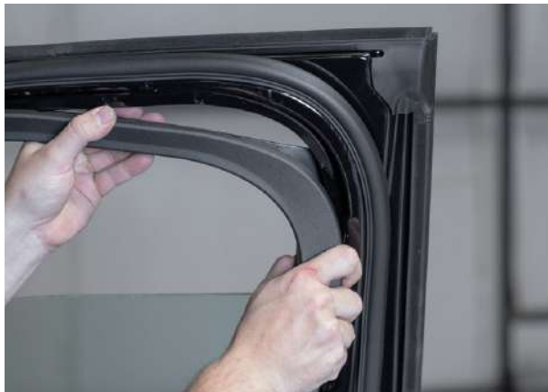
▲ Figure 44. Removing window trim
