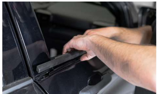
▲ Figure 22. Removing the outer window weatherstrip
