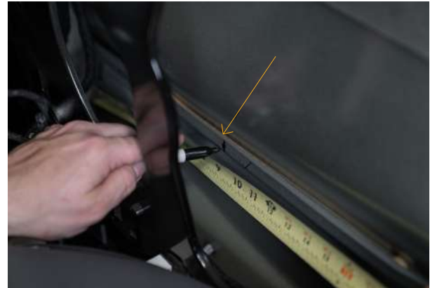
▲ Figure 48. Marking 9.5 inches towards the rear of the vehicle from the front of the crash bar
