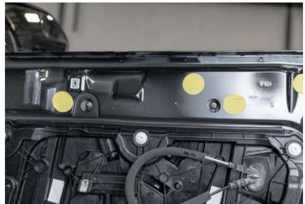
▲ Figure 38. Showing the window regulator mounting nuts
