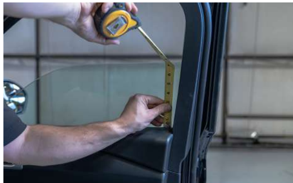
▲ Figure 32. Measuring the window height
