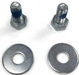
▲ Figure 12. Lower mounting bracket bolts and washers
