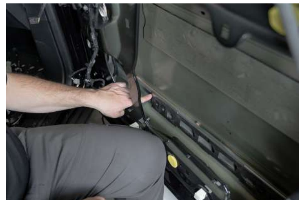
▲ Figure 50. Crash bar bracket and located in the door
