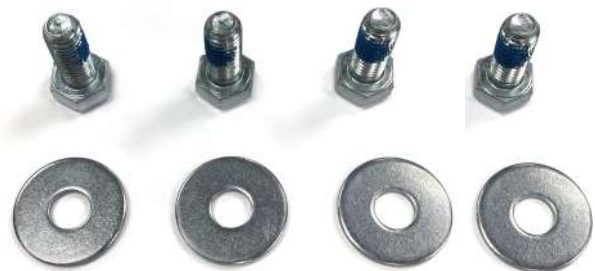
▲ Figure 9. M8 x 30 mounting bolts and washers
