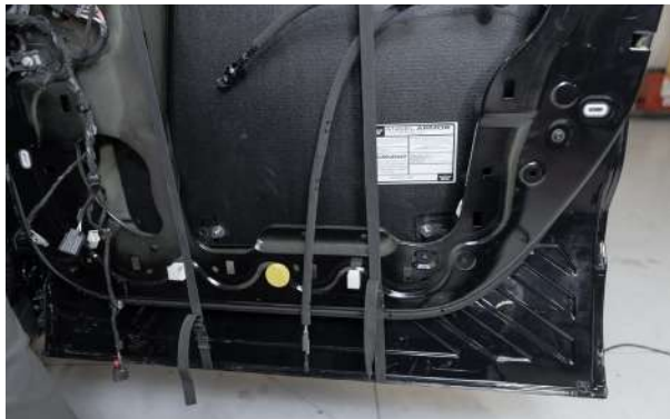
▲ Figure 54. The front, top crash bar bracket loosely installed
