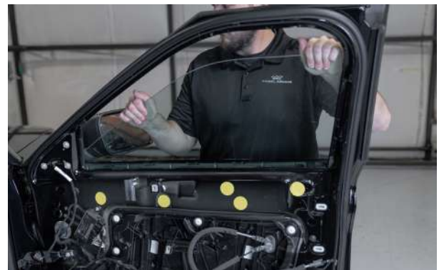
▲ Figure 34. Removing the window glass
