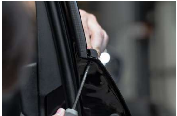
▲ Figure 21. Removing the back window weatherstrip screw
