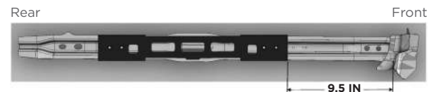
▲ Figure 49. Rendering of the crash bar mounting bracket showing location of the crash bar
