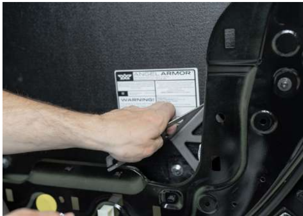
▲ Figure 56. Inserting Lower Mounting Bracket
