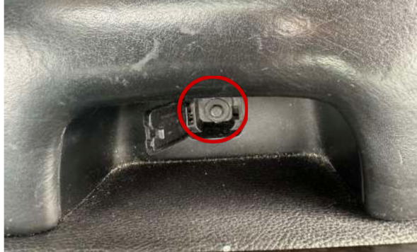
▲ Figure 21. Removing 7mm screw
