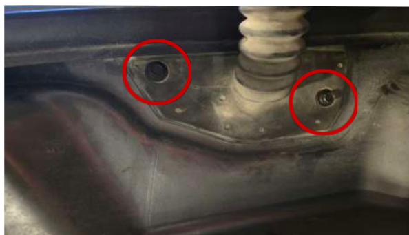
▲ Figure 25. Removing screws from the wire harness mount
