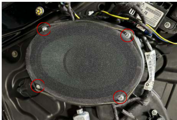
▲ Figure 22. Removing speaker using a torx T-20 screwdriver
