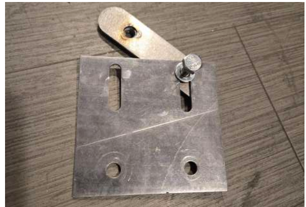
▲ Figure 31. Attaching one Pill Box Washer to the back of a Top Bracket
