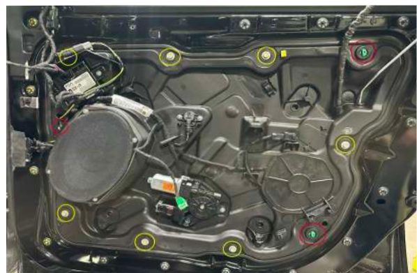
▲ Figure 23. Removing bolts around regulator panel. (yellow circle indicates sockets, red circle indicates torx)
