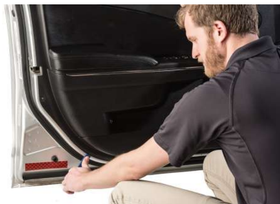
▲ Figure 28. Prying the door panel away from the door skin.
