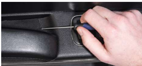
▲ Figure 25. Removing the armrest pocket trim cover.
