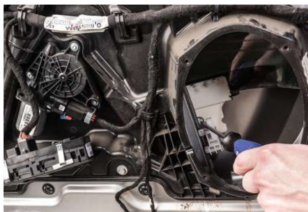
▲ Figure 31. Releasing the front window clip.
