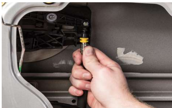
▲ Figure 35. Disconnecting the cable from the door handle mechanism.
