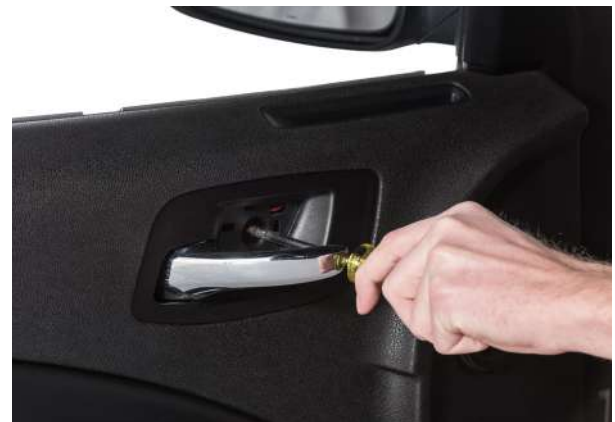
▲ Figure 24. Removing the interior door handle screw.
