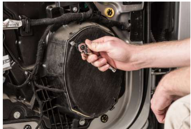
▲ Figure 30. Removing the speaker screws.
