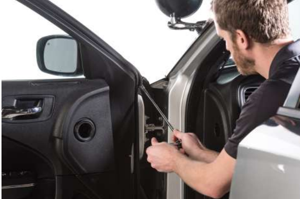
▲ Figure 20. Removing the front window weatherstrip screw.
