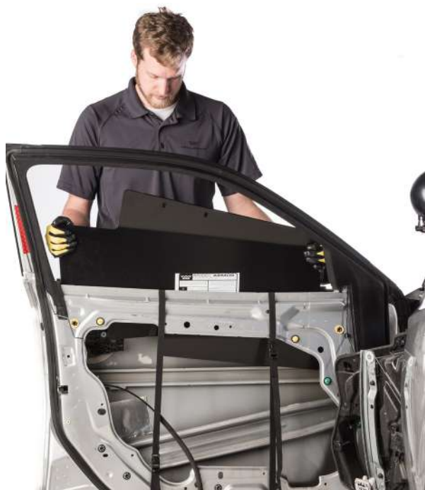
▲ Figure 39. Using the cradle created by the installation straps to lower the armor into the door.
