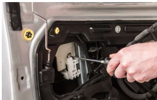
▲ Figure 33. Releasing the back window clip.
