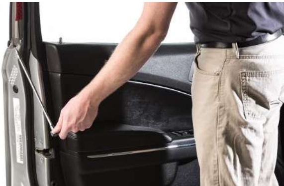
▲ Figure 21. Removing the back window weatherstrip screw.
