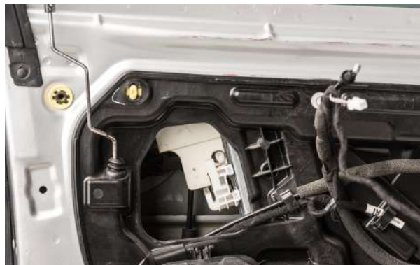
▲ Figure 32. Location of the window regulator access panel.
