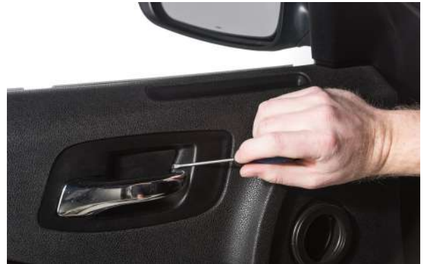
▲ Figure 23. Remove the interior door handle trim cover.
