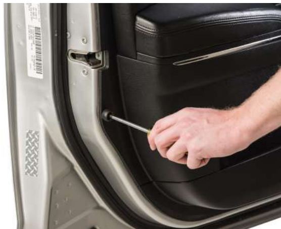
▲ Figure 27. Removing screw at bottom edge of the door panel.
