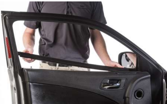
▲ Figure 22. Removing the outer window weatherstrip.
