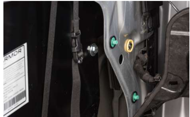
▲ Figure 41. The front, top crash bar bracket loosely installed.
