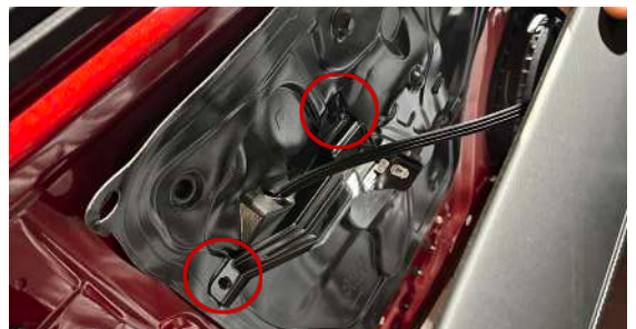
▲ Figure 26. Removing 2 screws on handle bracket
