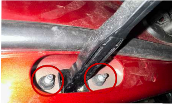
▲ Figure 42. Removing nuts from factory door stop
