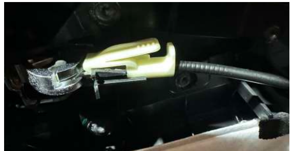
▲ Figure 25. Disconnecting door control panel wiring
