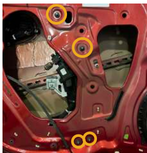
▲ Figure 28. Removing window regulator nuts
