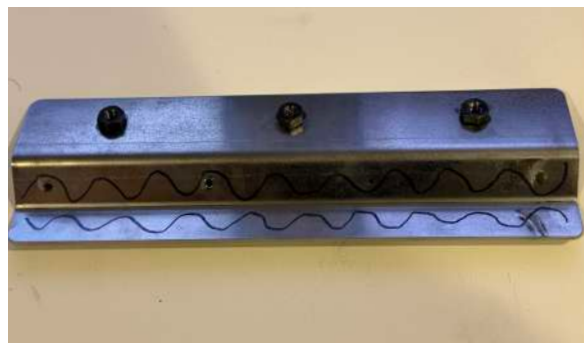
▲ Figure 40. Applying panel adhesive to upper section of the upper bracket
