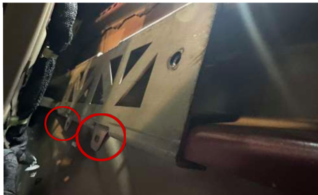
▲ Figure 35. Placing crash bar bracket on the crash bar
