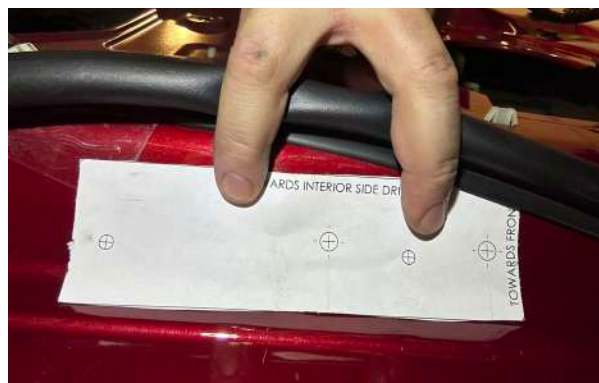
▲ Figure 34. Aligning drill template on the bottom of the door
