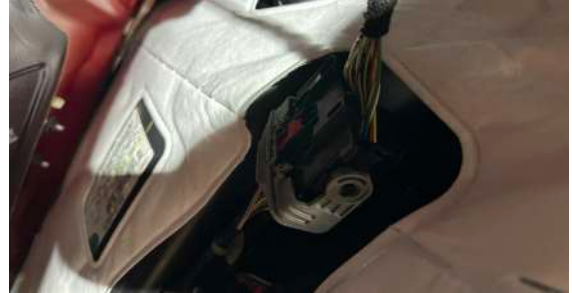
▲ Figure 24. Disconnecting interior handle cabler
