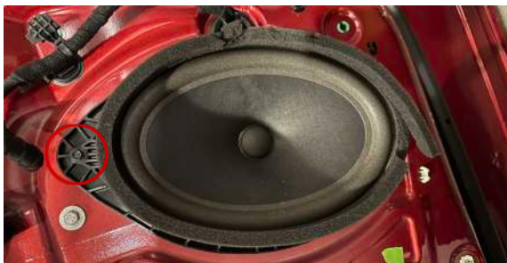
▲ Figure 27. Removing speaker screw
