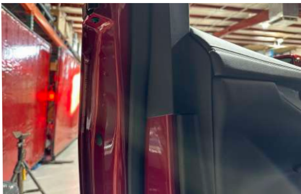
▲ Figure 31. Removing exterior trim
