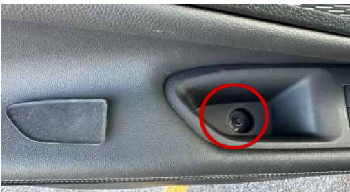
▲ Figure 23. Removing screw with 7mm socket
