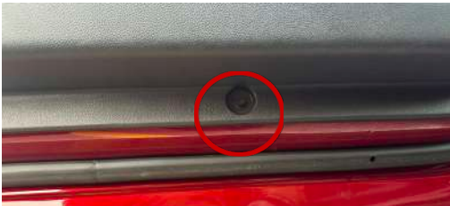
▲ Figure 22. Removing screw at the bottom of the door
