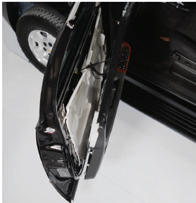
▲ Figure 9. Leaning open the interior door trim panel
