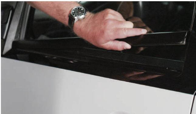
▲ Figure 11. Removing the outer window weatherstrip
