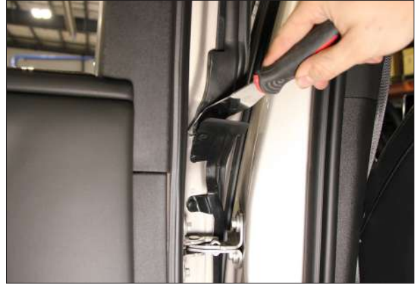
▲ Figure 8. Exposing the front Torx screw
