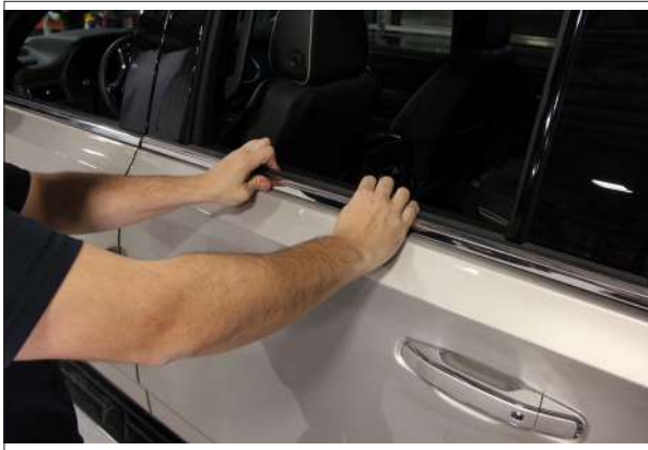
▲ Figure 16. Proper weatherstrip alignment
