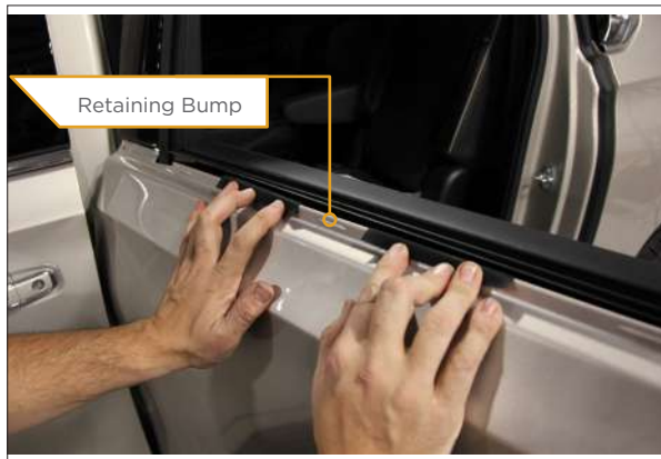
▲ Figure 14. Proper location of nylon folds
