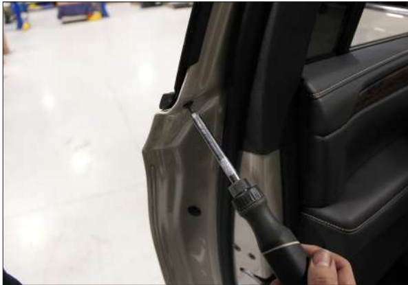
▲ Figure 7. Removing the rear Torx screw
