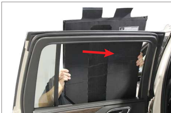
▲ Figure 12. Pushing panel forward while inserting panel
