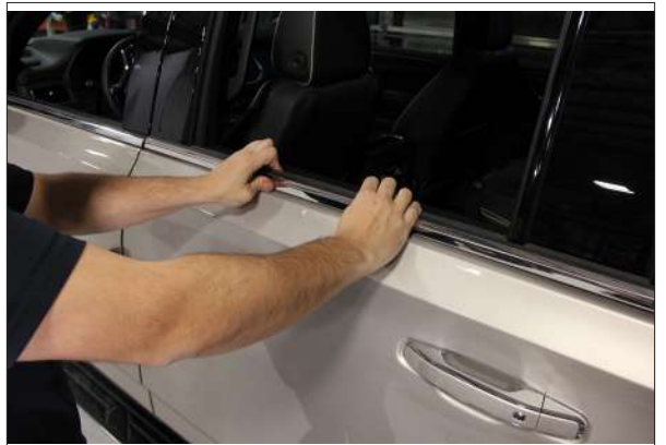
▲ Figure 10. Removing the weatherstrip
