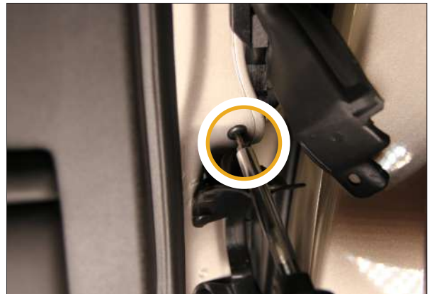
▲ Figure 9. Exposing the front Torx screw
