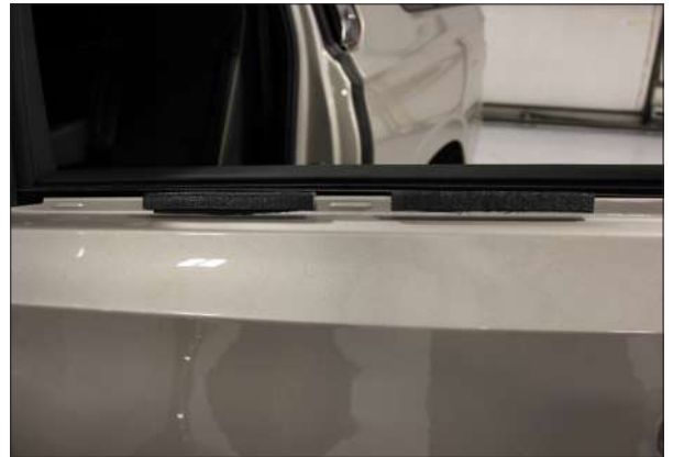
▲ Figure 15. Proper placement of Door Panel Grips
