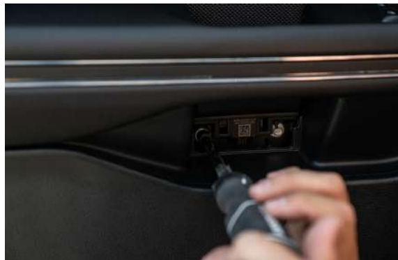
▲ Figure 14. Removing 8 mm panel mounting bolts
