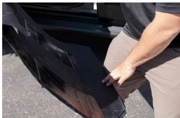
▲ Figure 22. Bending the ballistic panel
