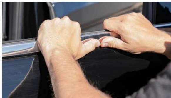
▲ Figure 21. Removing the window trim
