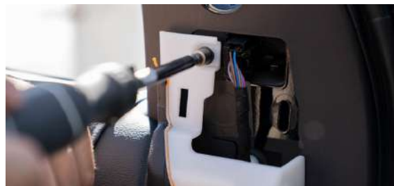
▲ Figure 16. removing the 7 mm mounting bolt
