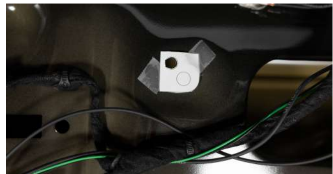
▲ Figure 37. Location of driver's side drill guide D
