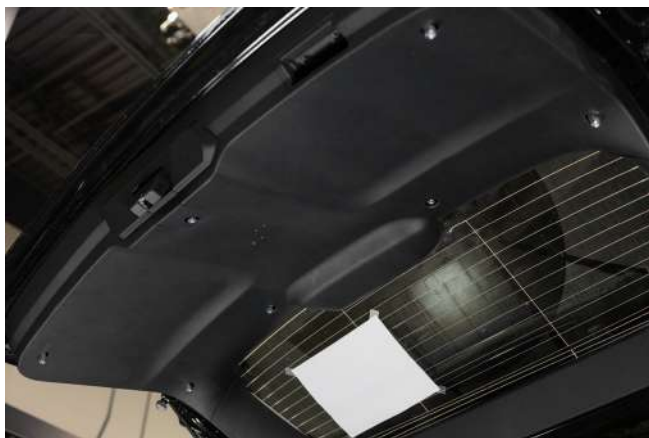
▲ Figure 38. Standoff locations once trim pieces are reinstalled
