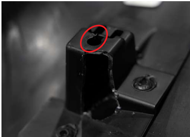
▲ Figure 32. Rivet housing after utility knife modifications
