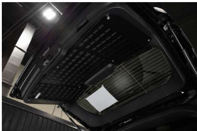
▲ Figure 40. Final armor placement once bolts are tightened
