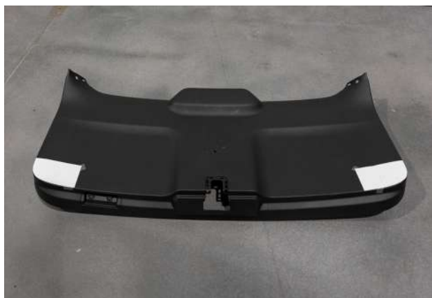
▲ Figure 28. Drill guides A (driver and passenger) aligned with bottom corners of hatch interior trim
