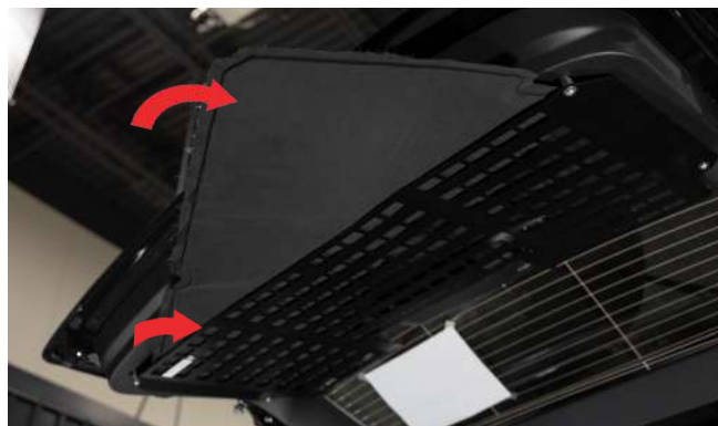
▲ Figure 39. Sliding ballistic panel between MOLLE panel and hatch trim
