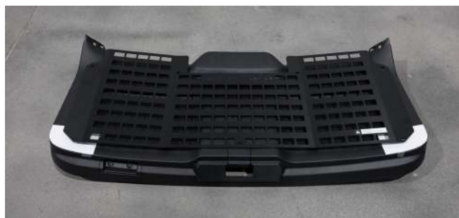
▲ Figure 30. Location of MOLLE panel when center punching remaining holes
