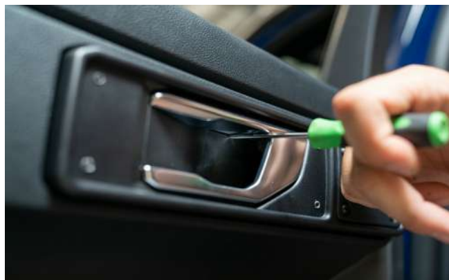
▲ Figure 13. Removing the trim cover.
