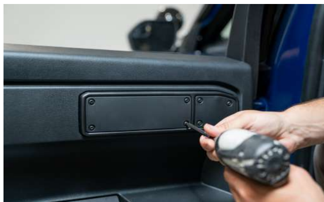
▲ Figure 12. Removing the four T20 screws.
