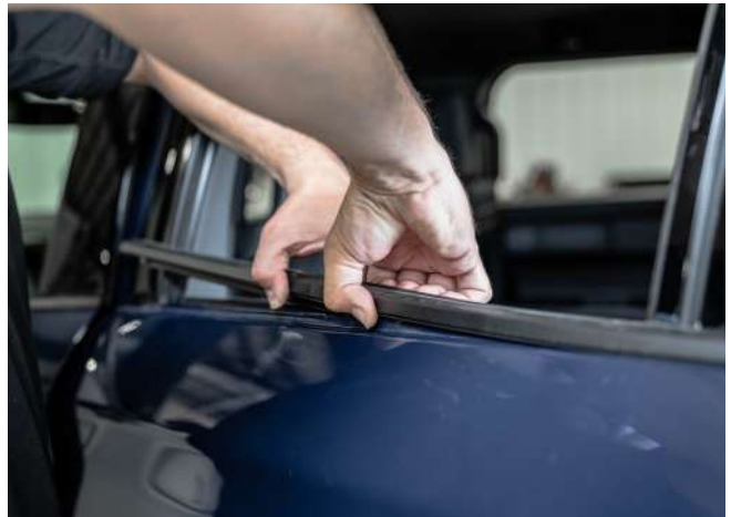
▲ Figure 10. Removing the window trim
