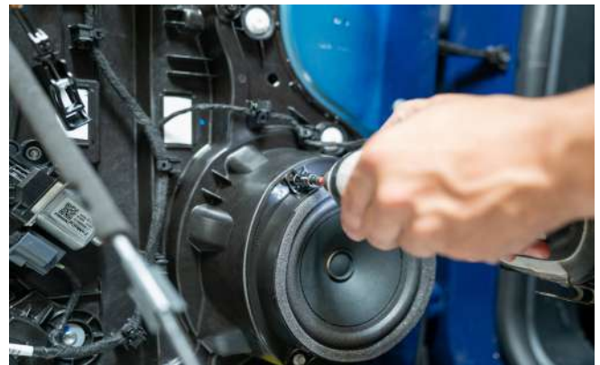
▲ Figure 18. Removing screws that hold the speaker.
