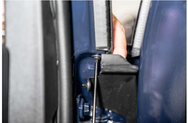
▲ Figure 9. Removing the Torx screw.
