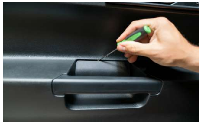
▲ Figure 15. Removing the trim cover.
