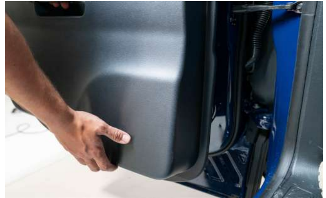
▲ Figure 17. Prying open the vehicle interior door trim panel
