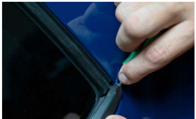
▲ Figure 11. Disconnecting rear weatherstrip clips.
