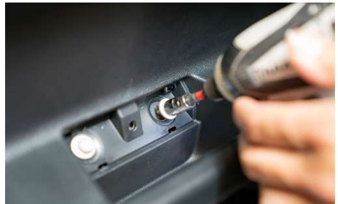
▲ Figure 16. Removing the 2 10mm screws.
