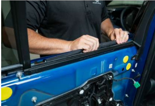
▲ Figure 23. Leaning back/pulling ballistic door panel toward exterior of the door.
