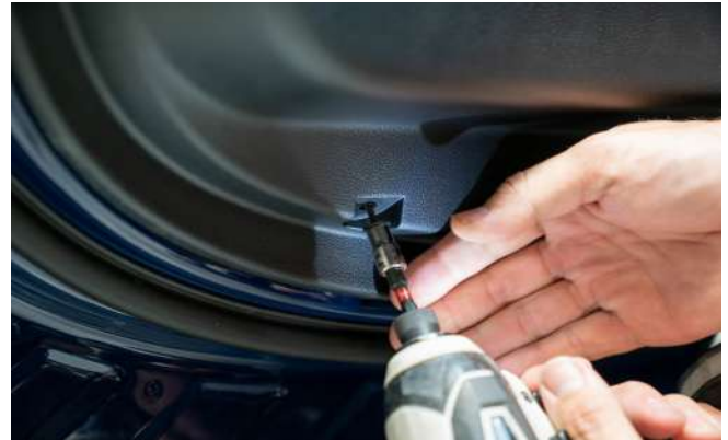
▲ Figure 14. Removing the 2 7mm screws.
