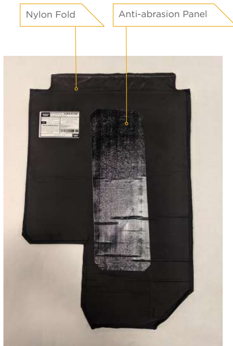
▲ Figure 1. Angel Armor Ballistic Door Panel (Level IIIA) for the Ford® Interceptor Utility Vehicle
