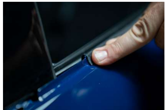
▲ Figure 24. Verifying the panel is 2 inches from the front of the window frame
