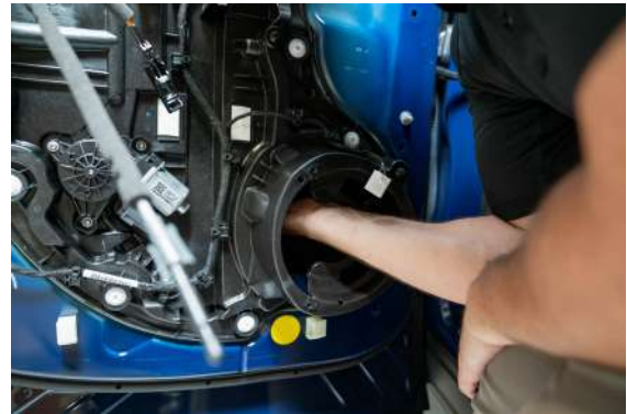
▲ Figure 20. Reaching into door to lead the bottom of the panel.
