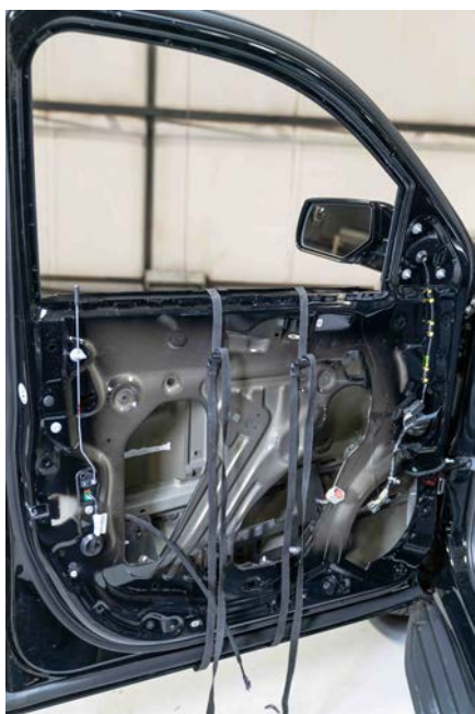
▲ Figure 51. Looping the installation straps around the door
