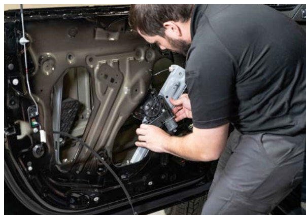
▲ Figure 39. Removing the window regulator
