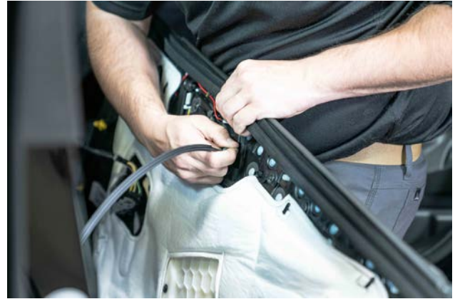
▲ Figure 30. Removing the door latch cable
