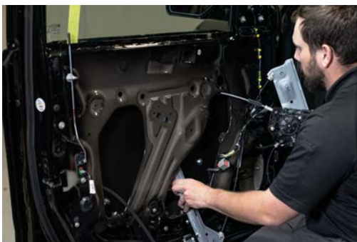
▲ Figure 63. Inserting the rear section of the window regulator.
