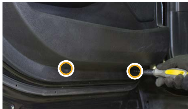
▲ Figure 27. Removing the door panel bolts
