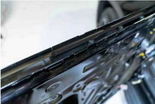
▲ Figure 59. Support Bracket aligned and installed
