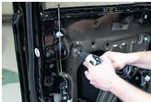
▲ Figure 64. Tightening the regulator mounting bolt
