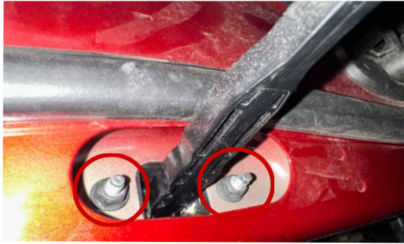
▲ Figure 42. Removing nuts from factory door stop
