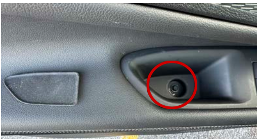
▲ Figure 23. Removing screw with 7mm socket
