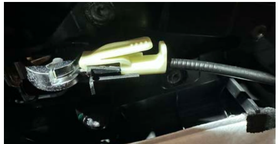
▲ Figure 25. Disconnecting door control panel wiring
