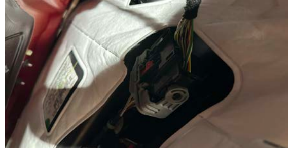
▲ Figure 24. Disconnecting interior handle cabler
