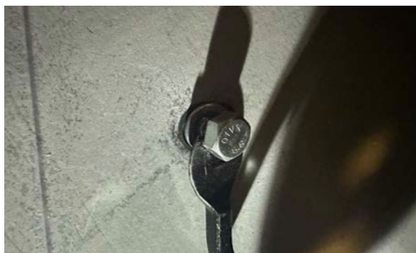
▲ Figure 39. Positioning hammer nut and bolt into middle crash bar
