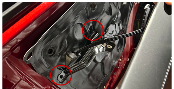
▲ Figure 26. Removing 2 screws on handle bracket
