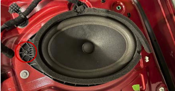
▲ Figure 27. Removing speaker screw
