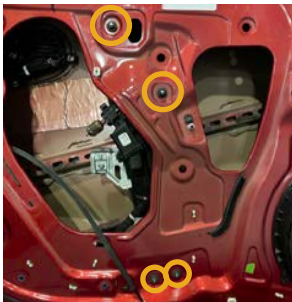
▲ Figure 28. Removing window regulator nuts
