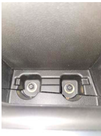
▲ Figure 24. Bolts revealed in handle pocket
