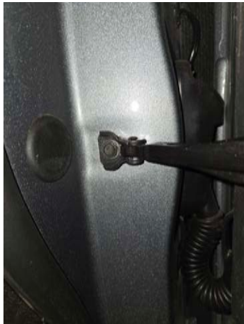
▲ Figure 22. OEM Check Strap mount
