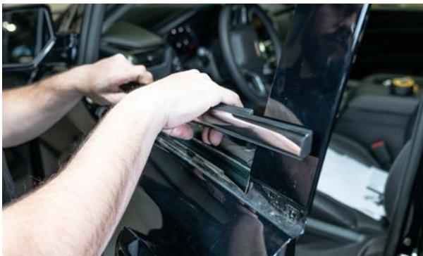
▲ Figure 24. Removing the outer window weatherstrip.
