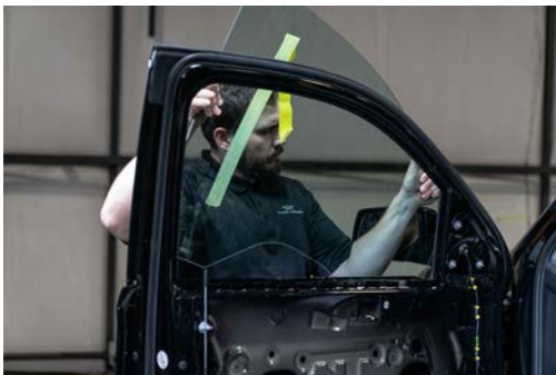
▲ Figure 77. Inserting the window glass into the window tracks.
