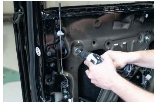
▲ Figure 72. Tightening the regulator mounting bolt.
