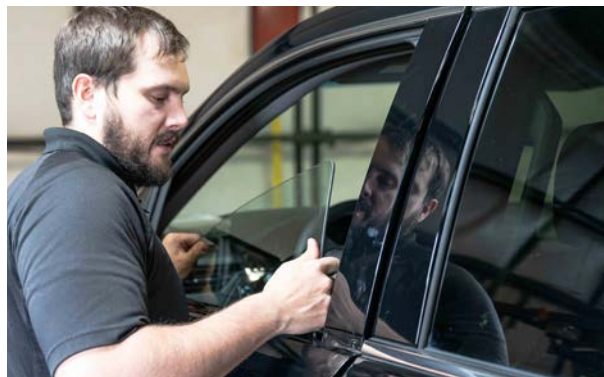
▲ Figure 39. Removing the window glass.
