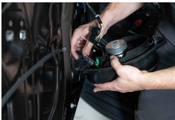
▲ Figure 31. Disconnecting the speaker harness.
