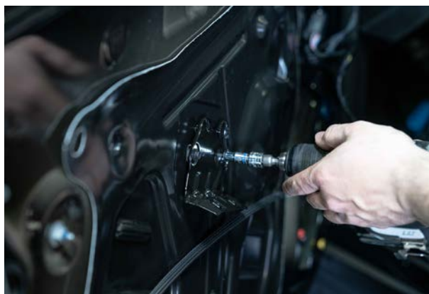
▲ Figure 32. Removing the door handle bracket.
