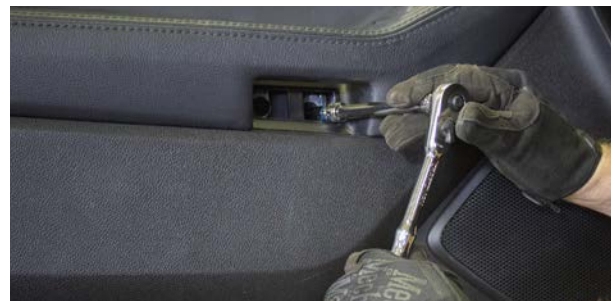
▲ Figure 26. Removing the armrest pocket bolts.
