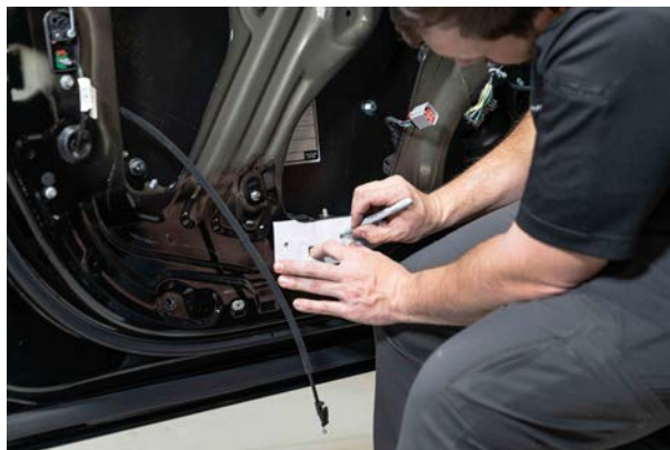
▲ Figure 59. Marking the hole locations using the template provided (appended to the end of this guide).
