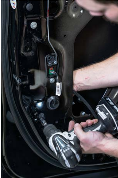
▲ Figure 76. Loosening the rear window track.
