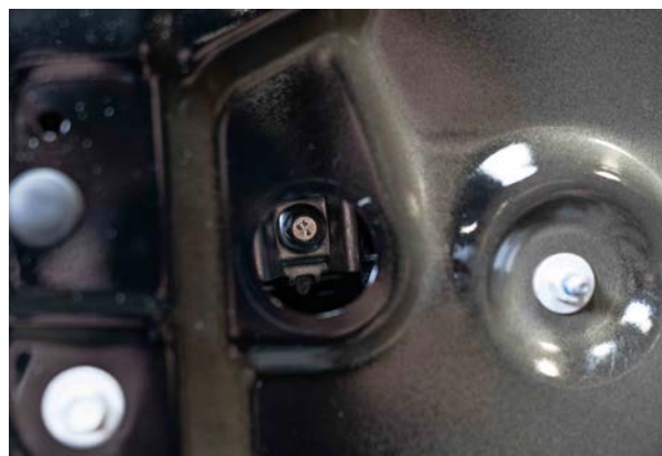
▲ Figure 37. Window regulator bolt head pictured through the inner door skin.
