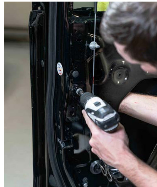
▲ Figure 75. Remove the upper window track bolt.
