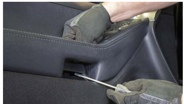
▲ Figure 25. Removing the armrest pocket trim cover.
