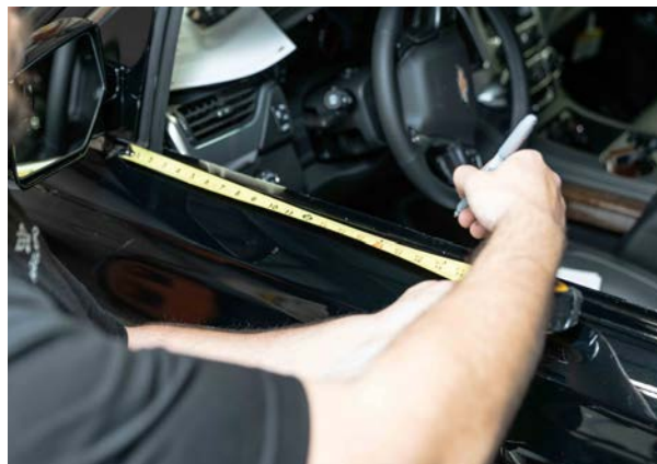
▲ Figure 45. Marking Bracket locations.
