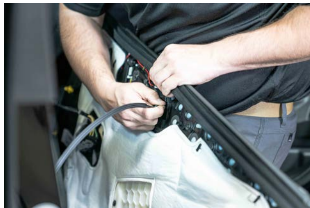
▲ Figure 30. Removing the door latch cable.
