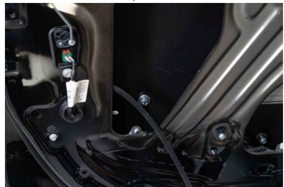
▲ Figure 58. The front, top crash bar bracket loosely installed.
