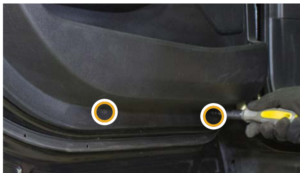
▲ Figure 27. Removing the door panel bolts.
