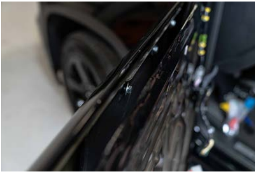
▲ Figure 61. Loosely installed upper mounting bracket..
