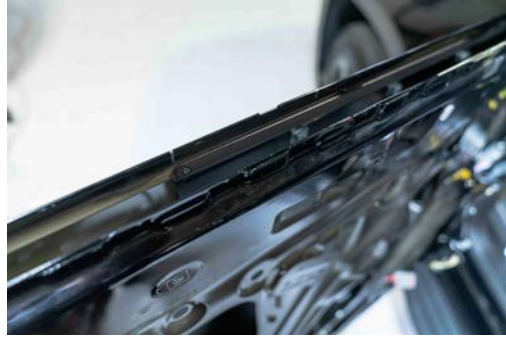
▲ Figure 66. Support Bracket aligned and installed.
