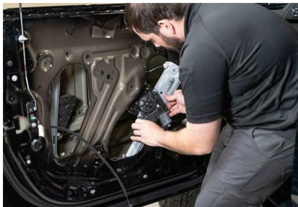
▲ Figure 42. Removing the window regulator.
