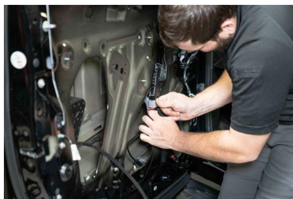
▲ Figure 40. Disconnecting the window regulator wiring harness.
