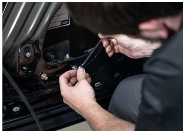
▲ Figure 60. Lower Mounting Bracket loosely installed.
