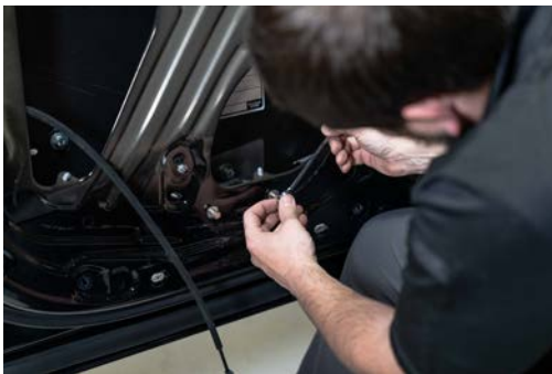
▲ Figure 73. Installing the lower mounting bracket.
