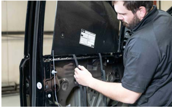
▲ Figure 55. Placing the armor into the door.
