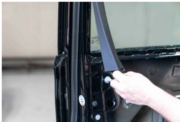
▲ Figure 35. Removing the window trim.
