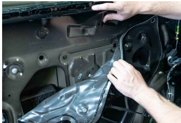
▲ Figure 33. Removing the weather seal.
