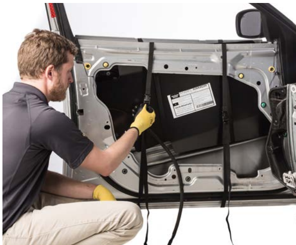
▲ Figure 54. Lowering the armor into the door using the installation straps.
