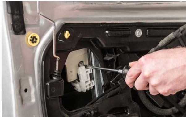
▲ Figure 42. Releasing the back window clip.
