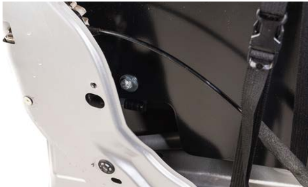
▲ Figure 53. The back crash bar bracket loosely installed.
