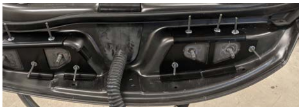
▲ Figure 25. Dry fitted brackets
