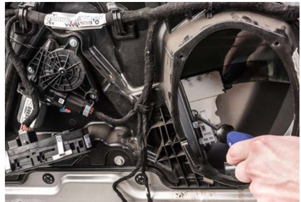
▲ Figure 40. Releasing the front window clip.
