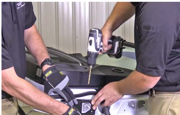
▲ Figure 24. Drilling the holes into the door.
