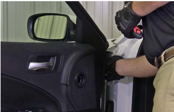
▲ Figure 18. Marking the hinges.
