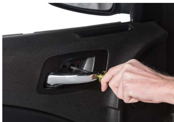
▲ Figure 33. Removing the interior door handle screw.
