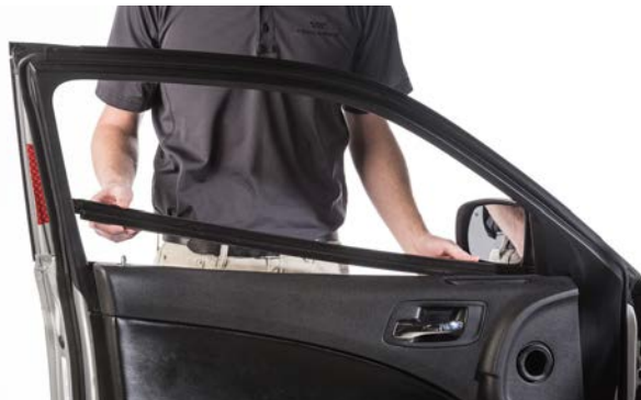
▲ Figure 31. Removing the outer window weatherstrip.
