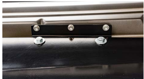
▲ Figure 57. Fully installed door mounting bracket. Looking up from the bottom of the door.
