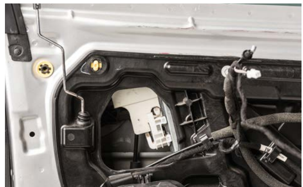
▲ Figure 41. Location of the window regulator access panel.
