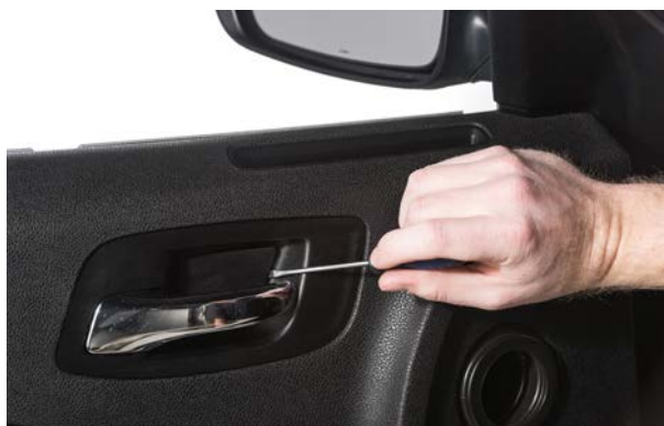
▲ Figure 32. Remove the interior door handle trim cover.
