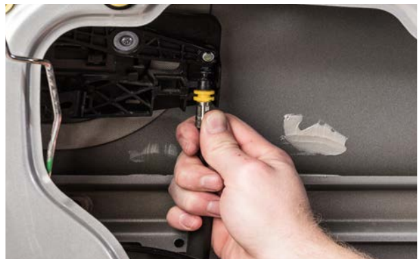
▲ Figure 44. Disconnecting the cable from the door handle mechanism.
