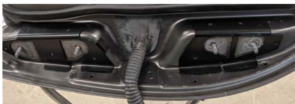
▲ Figure 23. Placing brackets on the door.
