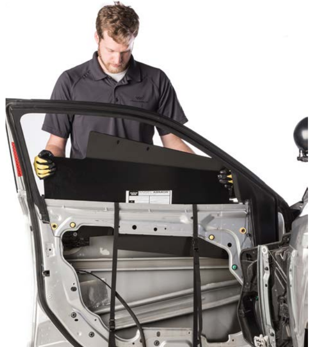
▲ Figure 48. Using the cradle created by the installation straps to lower the armor into the door.
