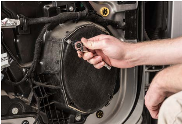
▲ Figure 39. Removing the speaker screws.
