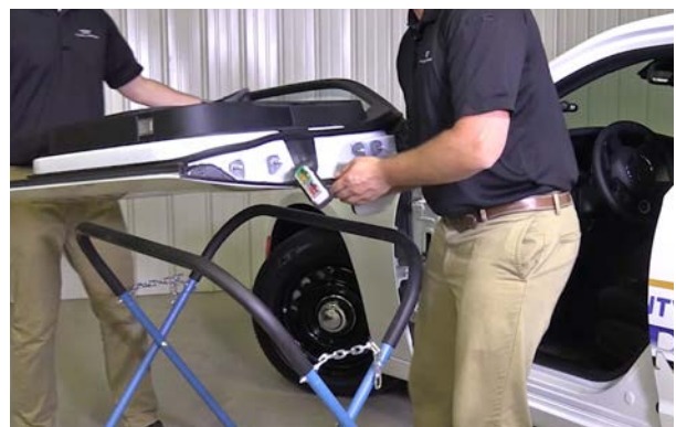
▲ Figure 21. Putting the door on the stand.
