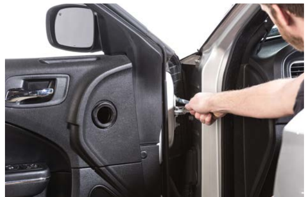
▲ Figure 20. Removing the upper door hinge bolt and nut.
