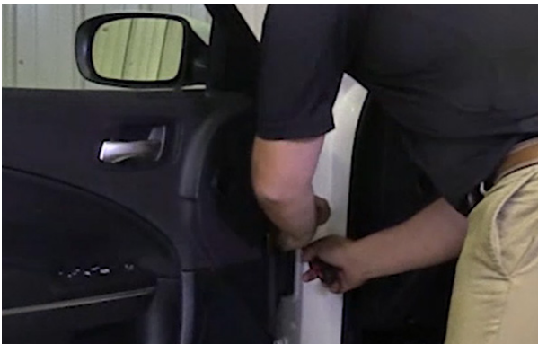
▲ Figure 19. Removing the wire harness.
