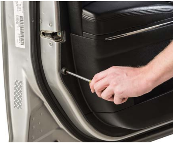
▲ Figure36. Removing screw at bottom edge of the door panel.
