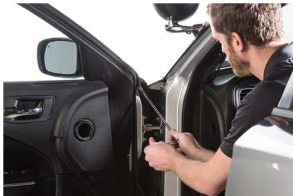
▲ Figure 29. Removing the front window weatherstrip screw.
