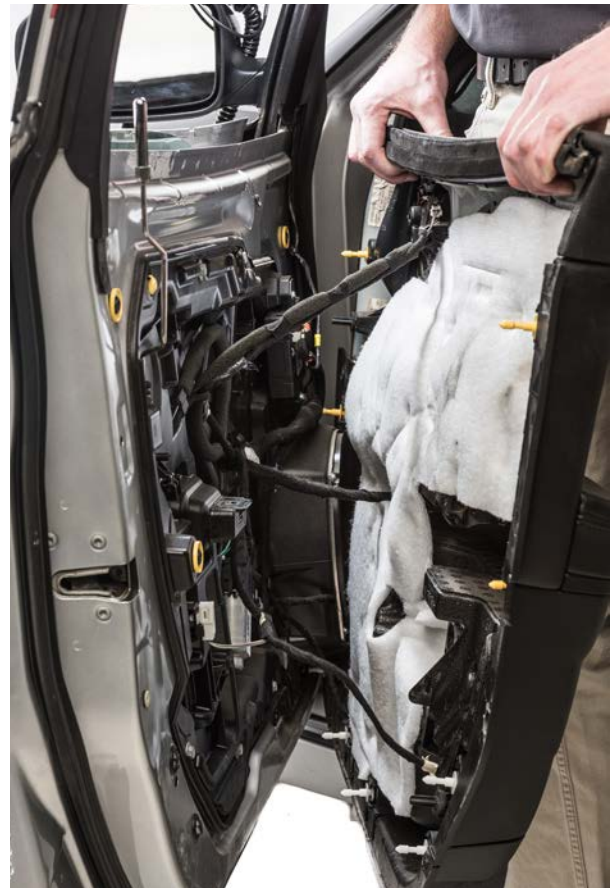
▲ Figure38. Tilting the door panel away from the door skin.
