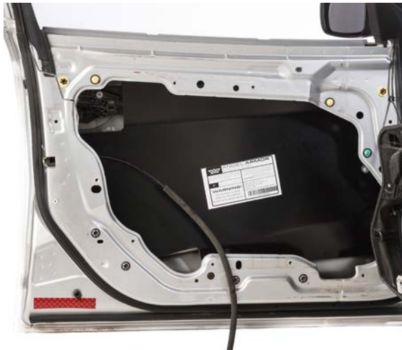
▲ Figure 56. The armor in its final position inside the door.
