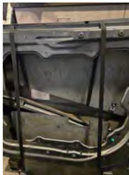
▲ Figure 28. Lowering Upper Armor halfway into the door
