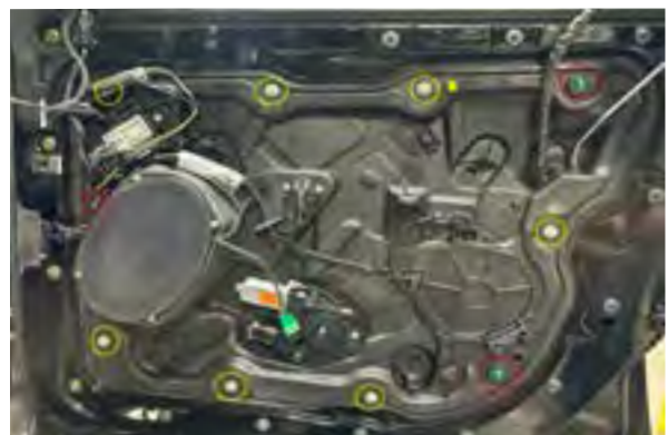
▲ Figure 23. Removing bolts around regulator panel. (yellow circle indicates sockets, red circle indicates torx)
