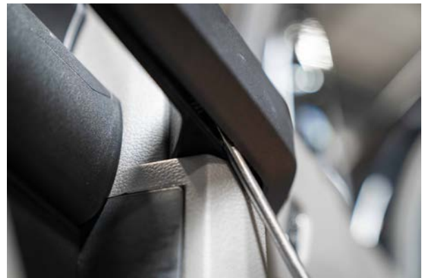
▲ Figure 21. Prying the trim panel loose
