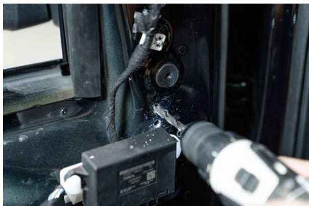
▲ Figure 44. Drilling the hole
