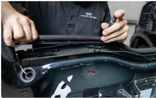
▲ Figure 31. Removing the outer window weatherstrip
