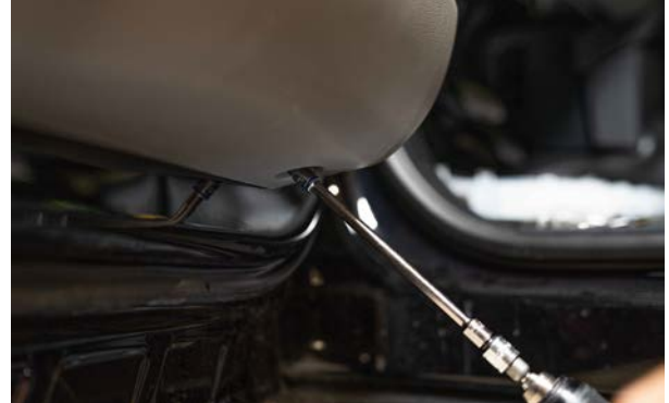
▲ Figure 25. Removing the lower panel bolts
