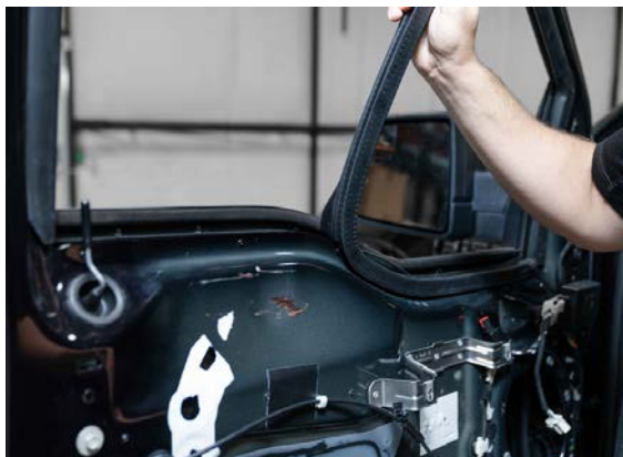
▲ Figure 32. Removing the inner weather stripping
