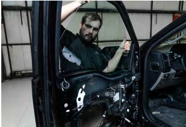
▲ Figure 37. Removing the window glass.
