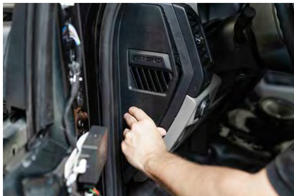
▲ Figure 46. Removing the trim piece.
