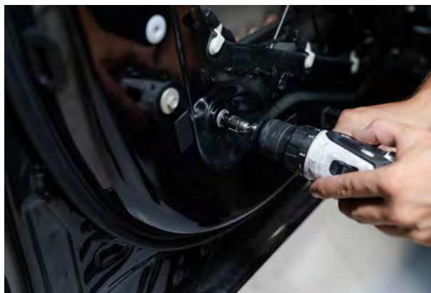
▲ Figure 42. Removing the window regulator mounting nuts.
