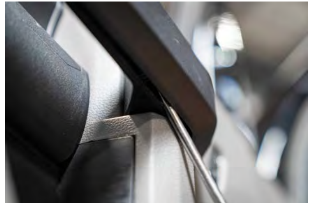
▲ Figure 21. Prying the trim panel loose.
