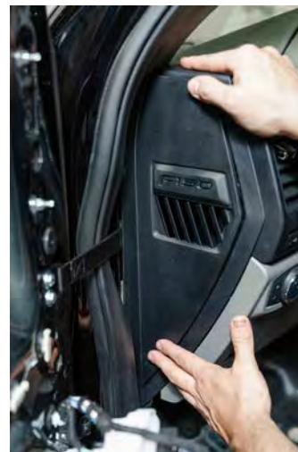
▲ Figure 54. Reinstalling the dash piece.
