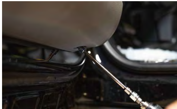
▲ Figure 25. Removing the lower panel bolts.
