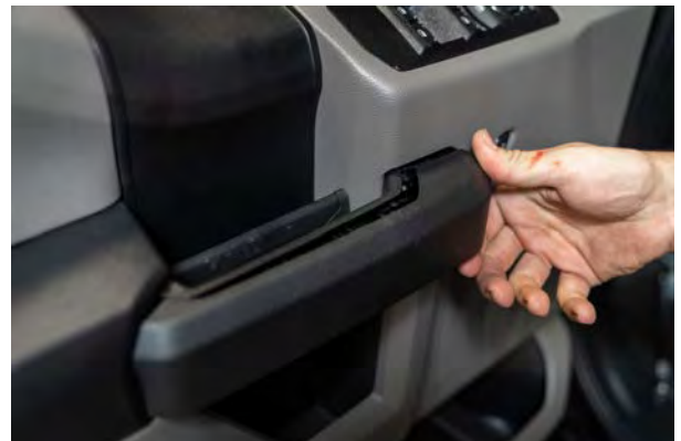
▲ Figure 22. Removing the handle panel.
