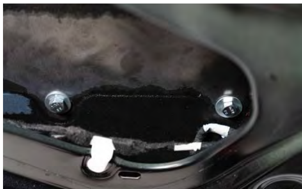
▲ Figure 76. Showing bolts that loosely install the crash bar.
