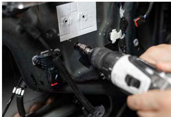
▲ Figure 43. Removing bolt from window regulator.
