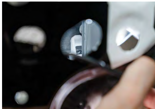
▲ Figure 34. Locating the window regulator clips.
