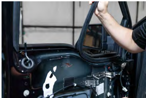
▲ Figure 33. Removing the inner weather stripping.
