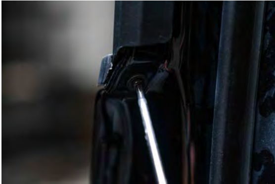
▲ Figure 29. Removing the back window weatherstrip screw.
