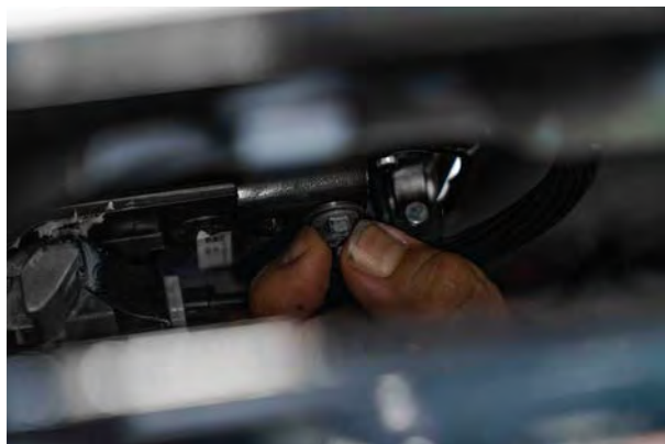
▲ Figure 60. Installing M6 nut with new fender washer.
