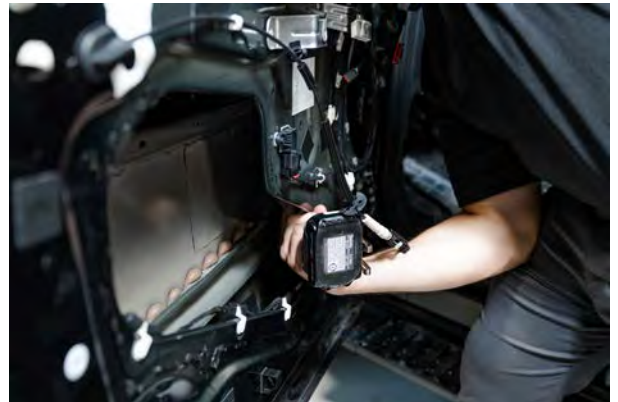
▲ Figure 69. Screwing in upper bracket.
