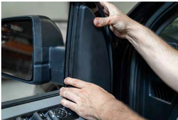
▲ Figure 19. Removing the trim panel.
