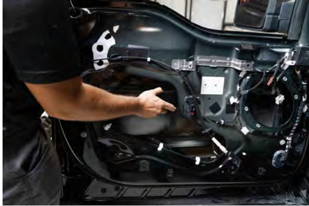
▲ Figure 66. Inserting the bracket into the door.
