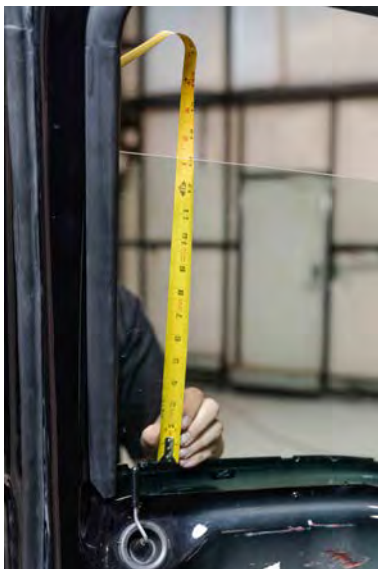
▲ Figure 32. Setting window height to 13 inches.
