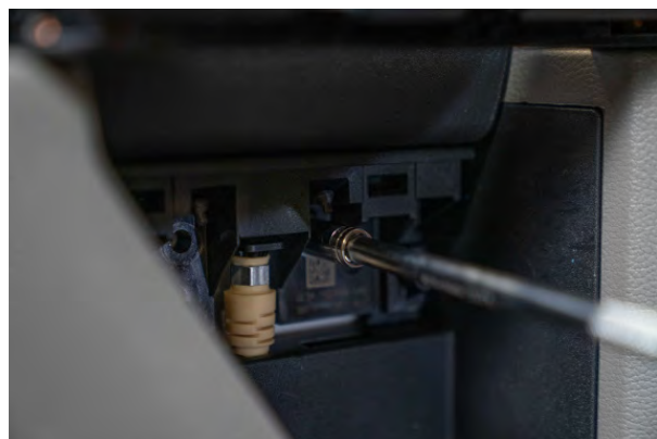
▲ Figure 24. Removing the interior door handle bolt.
