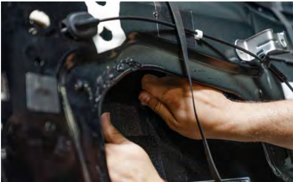
▲ Figure 77. Loosely attaching the mounting bracket.
