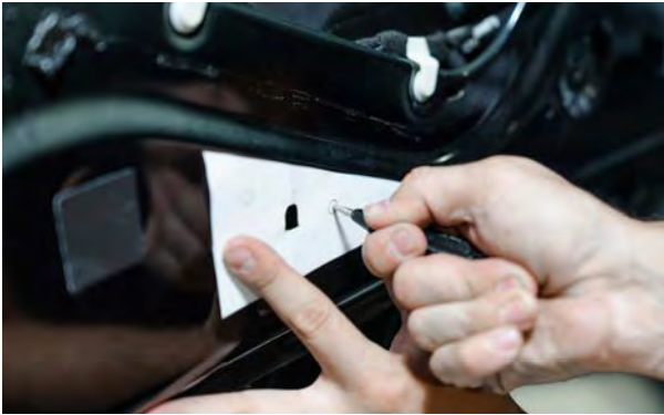
▲ Figure 80. Center punching the hole locations.
