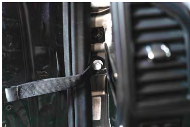
▲ Figure 52. Fastened check strap bracket to the dash frame.
