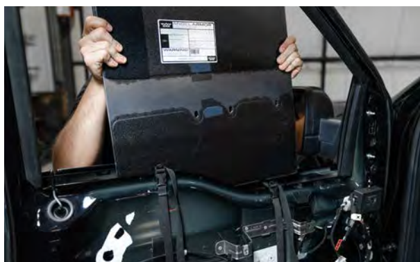
▲ Figure 74. Placing the armor into the door.
