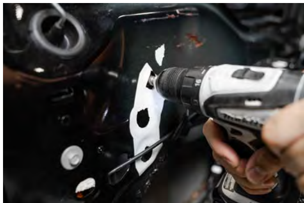
▲ Figure 41. Punching out the adhesive foam.
