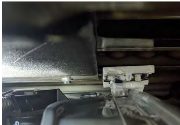
▲ Figure 81. Front window regulator clearance.
