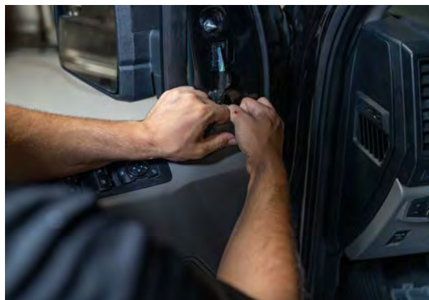
▲ Figure 26. Prying the door panel away from the door skin.
