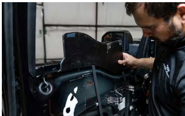
▲ Figure 75. Placing the armor into the door.
