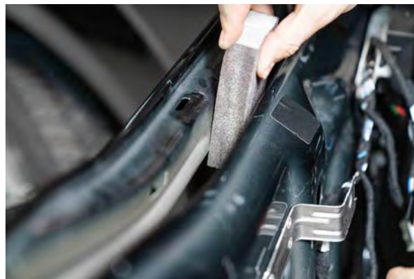
▲ Figure 57. Removing rust, primer and paint.
