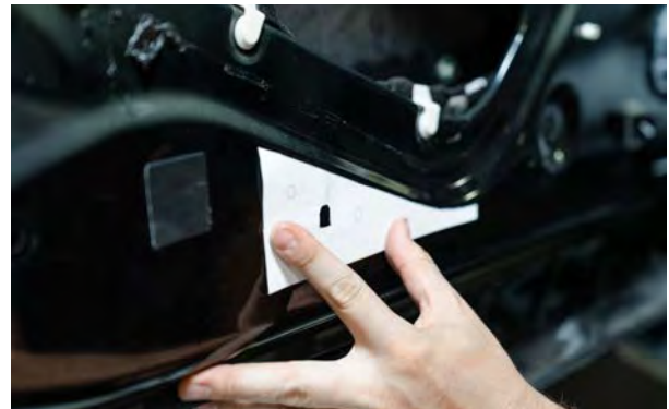
▲ Figure 79. Positioning the drill template.
