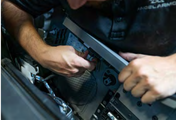
▲ Figure 27. Removing the door panel.
