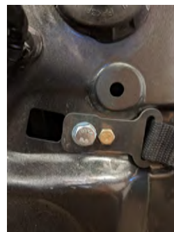
▲ Figure 45. Check strap mounting on the door.
