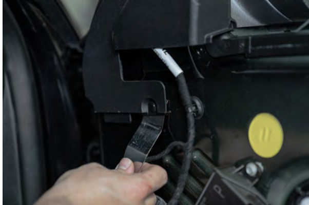
▲ Figure 42. Removing window trim from clips.
