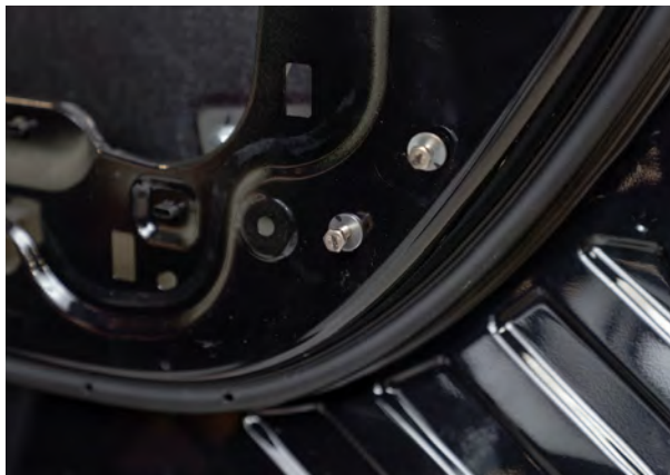
▲ Figure 56. Lower mounting bracket loosely installed.
