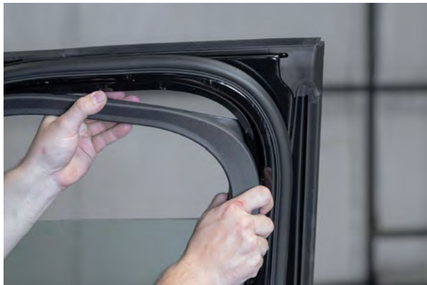
▲ Figure 43. Removing window trim.
