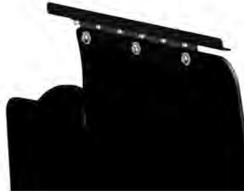
▲ Figure 57. Rendering of the armor and upper mounting bracket showing relative location and placement.
