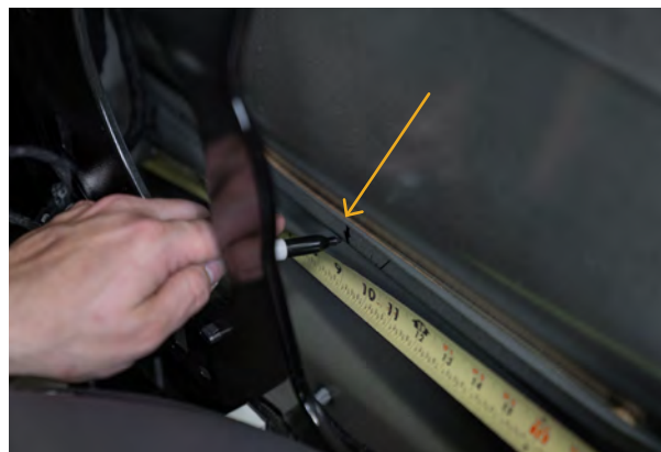
▲ Figure 47. Marking 9.25 inches toward the rear of the vehicle from the front of the crash bar.
