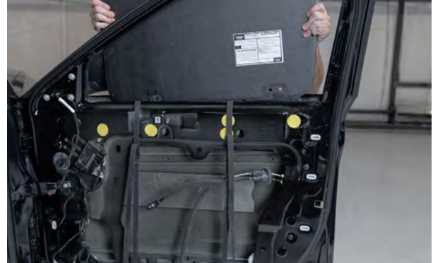
▲ Figure 51. Placing the armor into the door.
