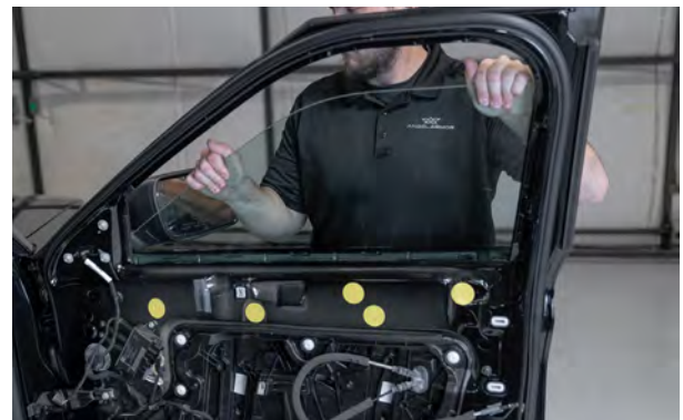
▲ Figure 33. Removing the window glass.
