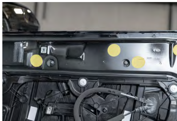
▲ Figure 37. Showing the window regulator mounting nuts.
