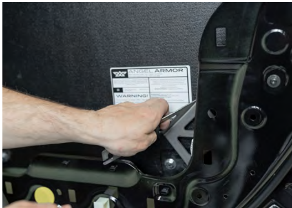
▲ Figure 55. Inserting Lower Mounting Bracket.
