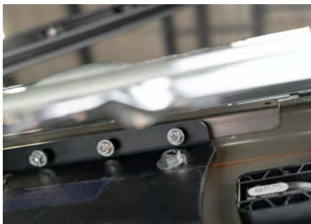
▲ Figure 62. The sheet metal screws installed into the door.
