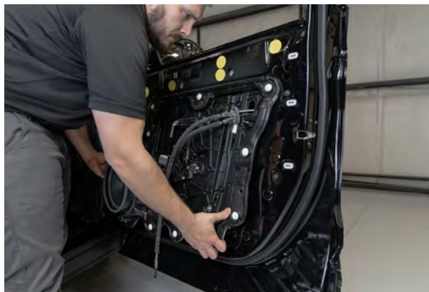
▲ Figure 38. Removing window regulator panel.
