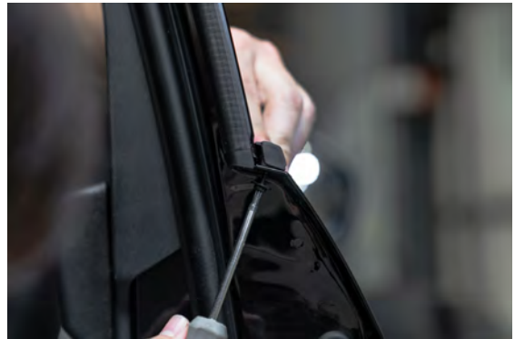
▲ Figure 20. Removing the back window weatherstrip screw.
