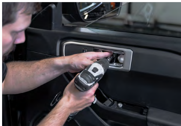
▲ Figure 23. Removing the interior door handle bolt.
