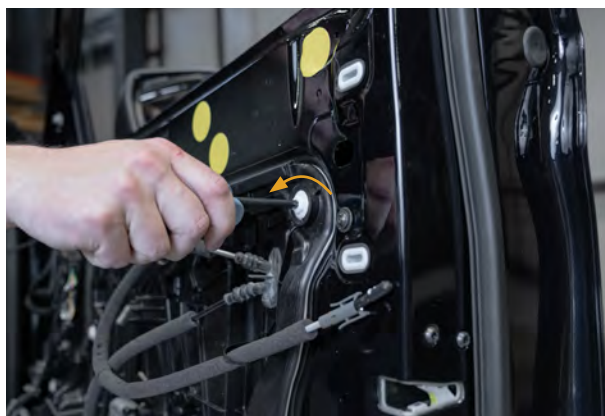
▲ Figure 35. Rotating Torx Clips.
