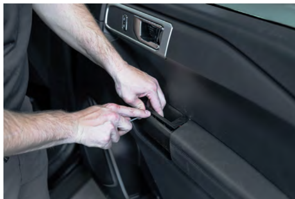
▲ Figure 24. Removing the interior door handle bolt.
