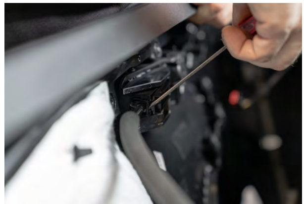
▲ Figure 29. Unclipping the door latches.
