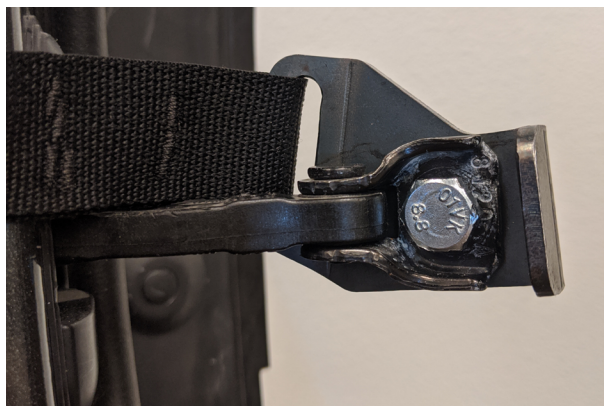
▲ Figure 46. Check strap orientation on A-pillar.
