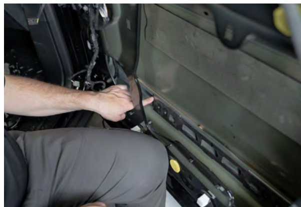
▲ Figure 49. Crash bar bracket and located in the door.
