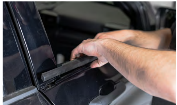
▲ Figure 21. Removing the outer window weatherstrip.
