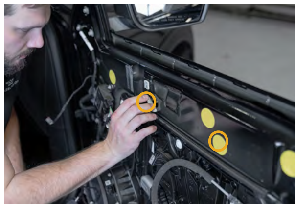
▲ Figure 36. Removing the adhesive patches.
