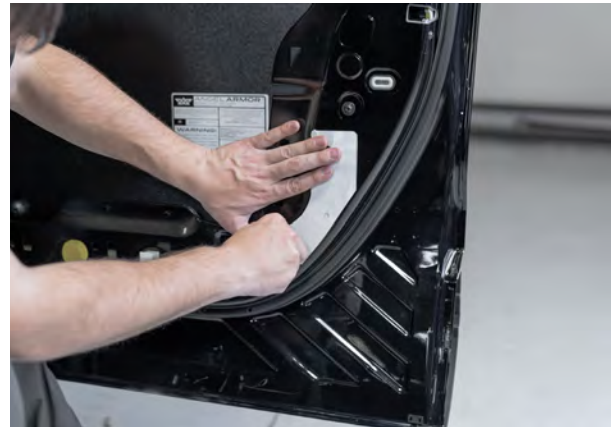
▲ Figure 54. Marking the hole locations using the template provided (appended to the end of this guide).
