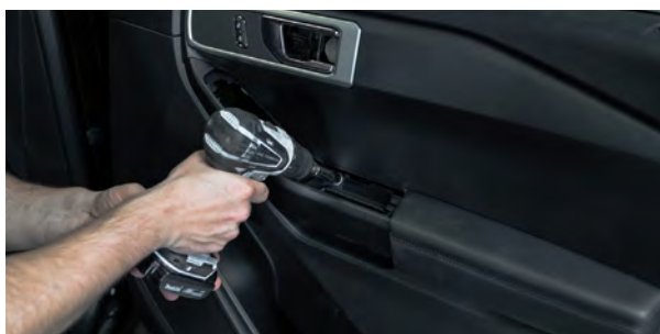
▲ Figure 25. Removing the armrest pocket bolts.
