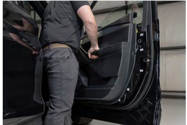
▲ Figure 28. Removing the door panel.
