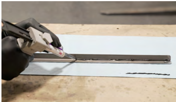
▲ Figure 59. Applying panel bond to support bracket.
