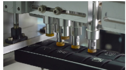
Panel buttons cycled 1.2 million times
