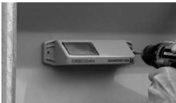
2. Assemble two (2) provided rivets through the drilled holes and install them using a rivet gun.
