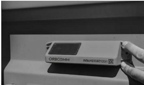
3. Press firmly on both mounting flanges of the CT 1000 (7 kg (15 lbs) for 10 seconds) to bond the tape to the asset.
