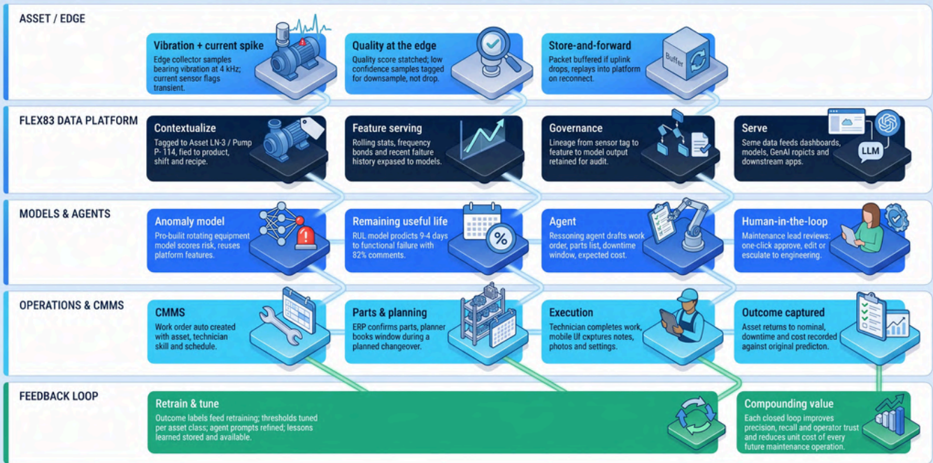
Figure 5.4 — Predictive maintenance traced end-to-end on Flex83: a single industrial data platform binds field signals to a work order, captures the outcome, and learns from it. Source: IoT83 reference deployment patterns, 2026.
