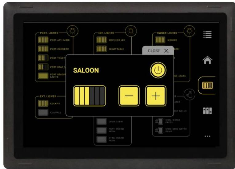
**⚠** If the HUB, for an undetermined reason, becomes inoperative, the variation of light intensity continues according to the **last values stored locally**, which allows the lights to remain usable but the adjustment is temporarily inoperative.
