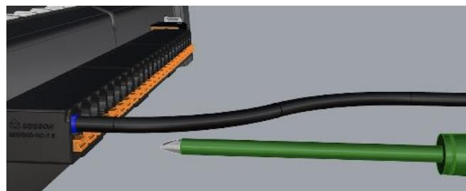
To ensure a reliable and vibration-resistant connection, all stranded conductors must be terminated with a crimped ferrule (metal end sleeve) before being inserted into the Degson push-in terminals. Bare stripped wire shall never be inserted directly into the connector. The ferrule must be crimped using an approved tool and fully seated into the spring-clamp mechanism to guarantee proper electrical contact and long-term mechanical retention.
