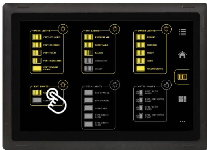
You can activate each consumer individually by clicking on each of the digital buttons associated with the different Powerail outputs (depending on the boat's configuration). Once the action is performed, the HUB analyzes it and sends the command (on or off) to the relevant Powerail(s). The Powerail(s) then sends back the output status to change the color of the corresponding button in the embedded application.
