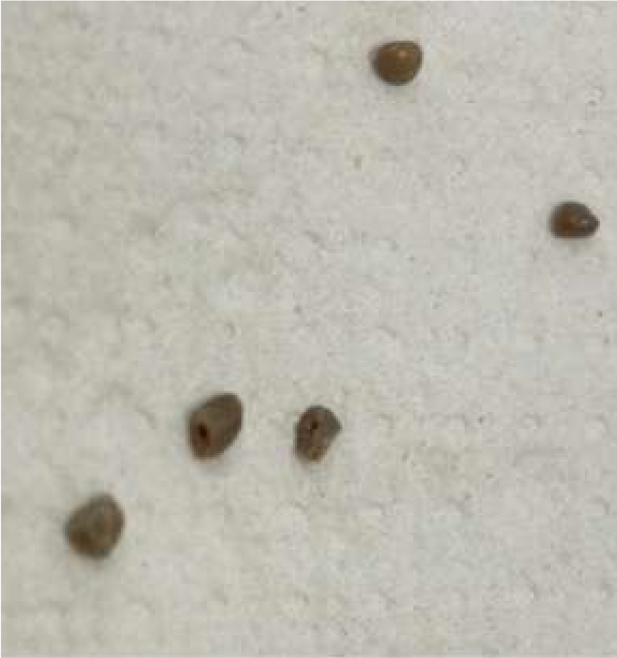
Image 31: Cross sections of unwashed post-consumer duvet pellets
