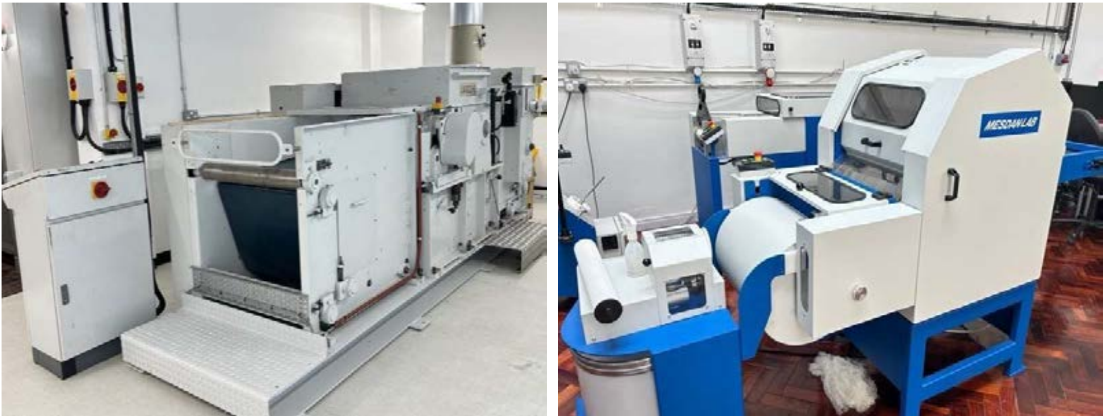
Image 27: Laboratory-scale Laroche Cadette tearing machine (left) and Mesdan carding machine (right)
