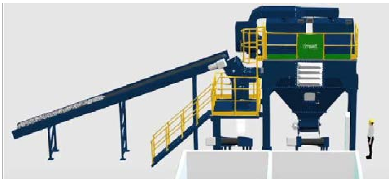
Image 16: Zigzag Air Classifier, provided by trial partner Impact Air Systems
