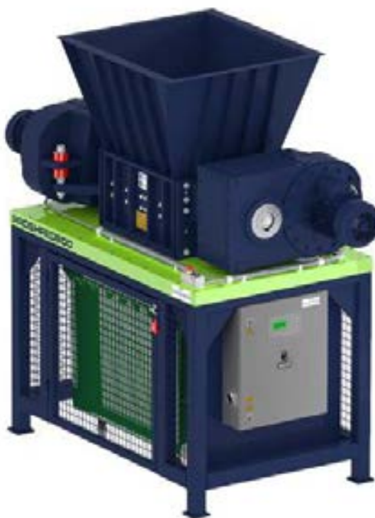
Image 12: Twin-shaft shredder, Proshed 800
