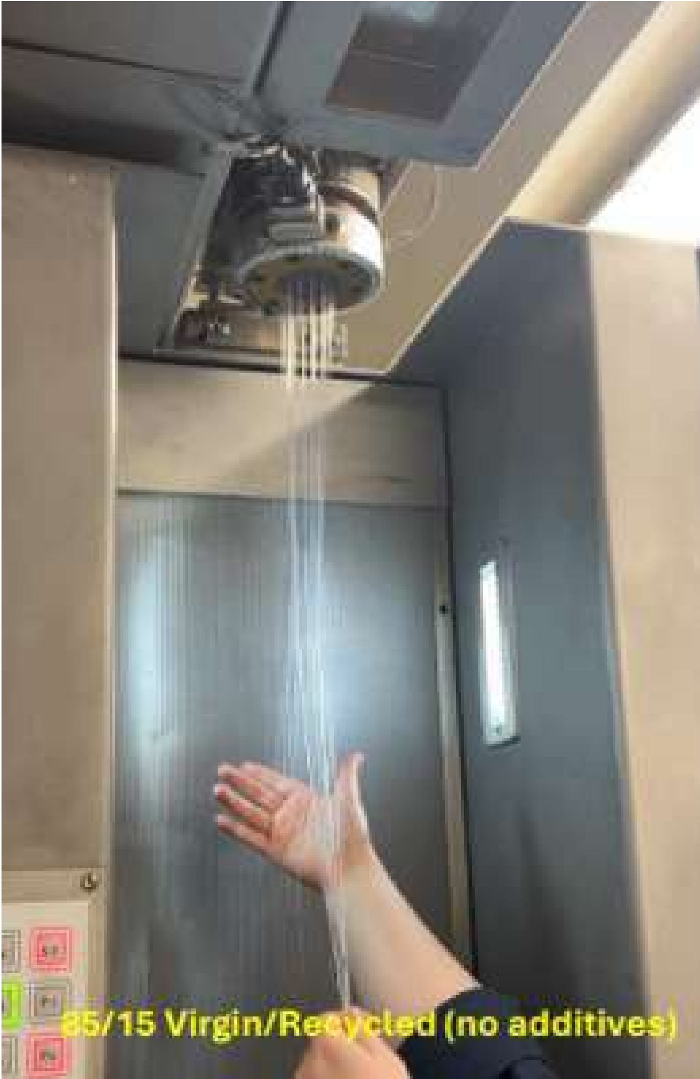
Image 33: 85% virgin polyester 15% recycled yarn extrusion, no master-batch
