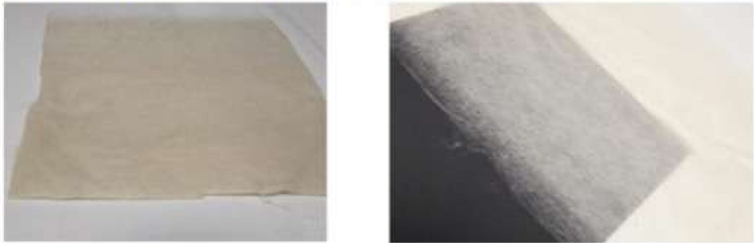
Example fibre web products produced at two fibre diameters with different gsm
