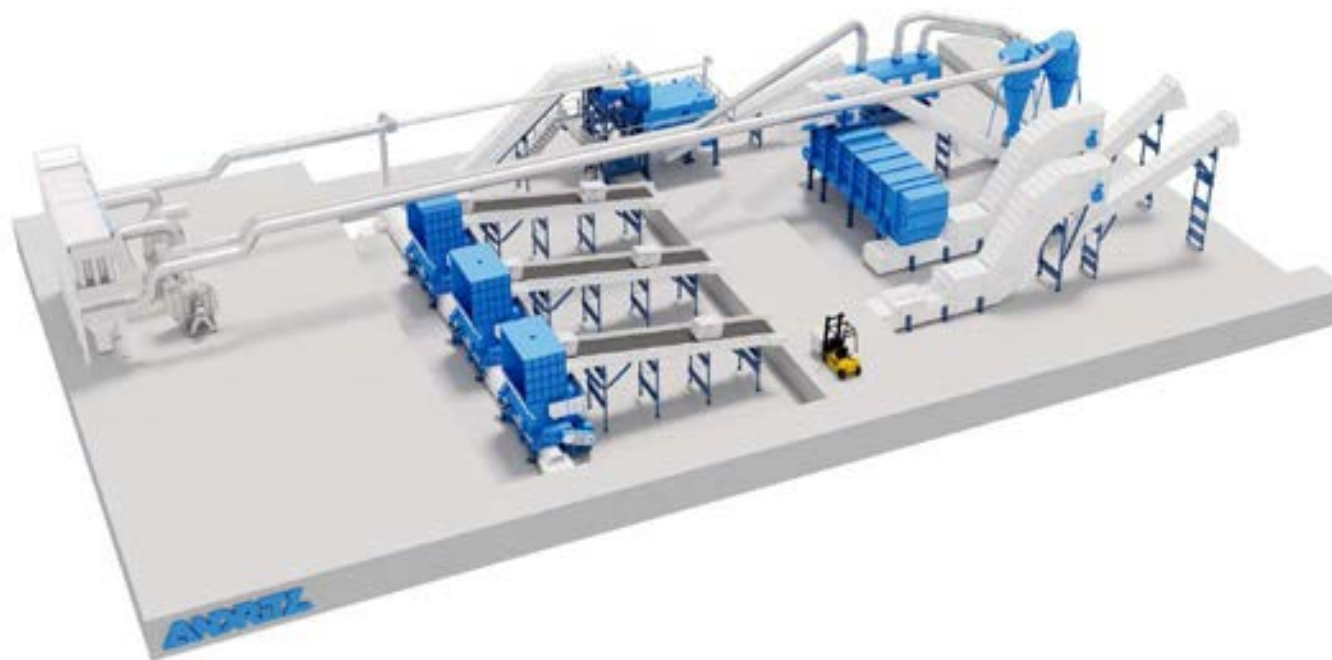
Figure 35: Exemplary textile waste conditioning system'
