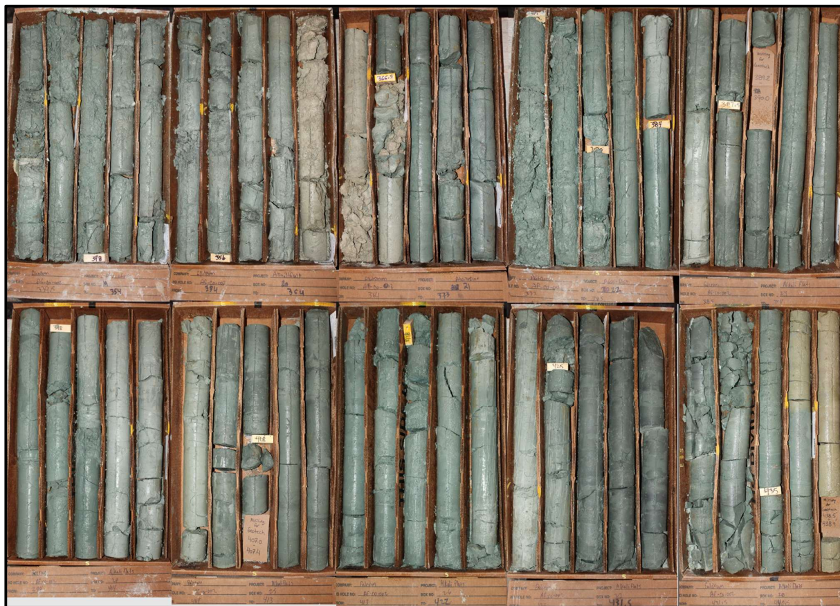
Figure 6. CORE OF SEIBERT FORMATION CLAYSTONE (AF3-CO2, 330ft - 440ft)
