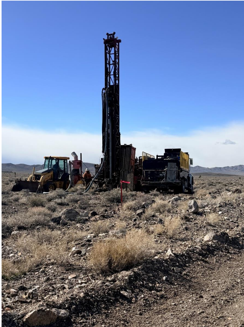
Figure A - 2 Active reverse circulation drilling observed during the site inspection.
