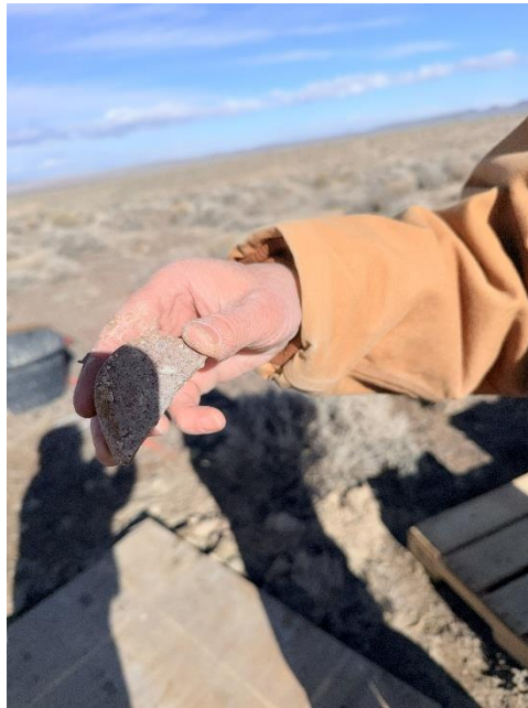
Figure A - 7 Claystone core.
