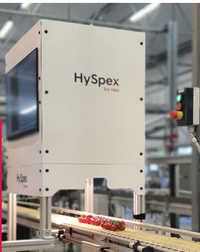
Figure 1: A compact HSI solution comprising hyperspectral instrumentation, illumination, and real-time quality grading output on an integrated screen. This image is from an early-stage demo setup at the customer site.
