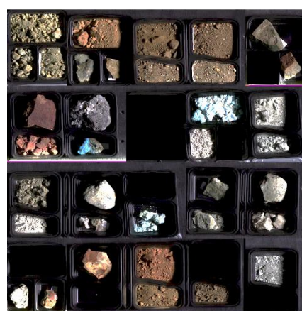
Figure 1. Sample-based spectral library. The 36 samples (left) collected onsite were analysed and characterised in the laboratory using both hyperspectral and traditional means. The samples were then grouped in clusters according to their common geochemical data. The spectral library (centre) was build using the reflectance from the clustered materials (C1-C7). The automated classification using ReSens+ (right) shows that the spectral cluster classes can be used to identify the samples. The library was later used to identify the materials/clusters on the mine face. ReSens+ is a software application by the German start-up rad. Data Spectral Analytic UG (limited).
