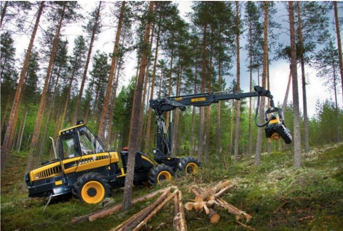
Application: tree harvesting, paired with a forwarding vehicle to remove the logs.
