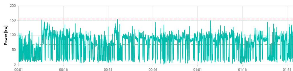
Figure 13. Power (kW) versus time (h) for Fendt 820, seedbed activity.
