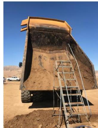
After MRA treatment the payload increased at least 20%. And the ease to clean the remaining of buildup also was considerable, metal surface shows very good performance (versus buildup formation) during treatment.
