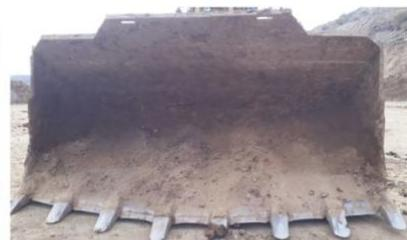
Slipcoat MRA was utilized at truck bodies and loader buckets, applied frequently at first time to form the non-stick barrier (to penetrate the metal surface as much as possible) and then increasing the application every 3 or 5 trips, until perform the MRA application 2-3 times per 12 hours shift.
