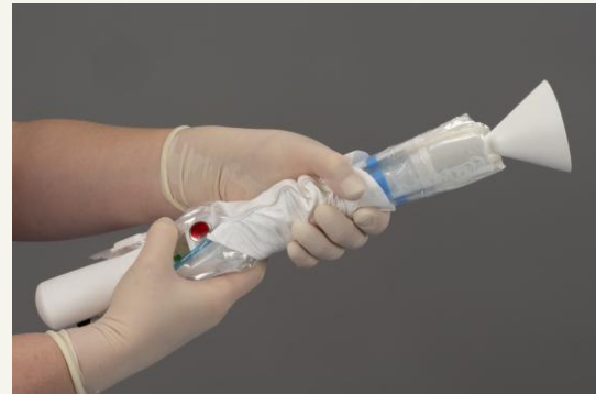
Figure 35 Pull back firmly on the fastening band to expose the sleeve
