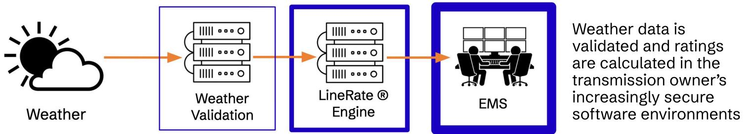
Transmission Owners typically place the LineRate Engine within their high-security SCADA environment, while others may place it in their corporate environment.
