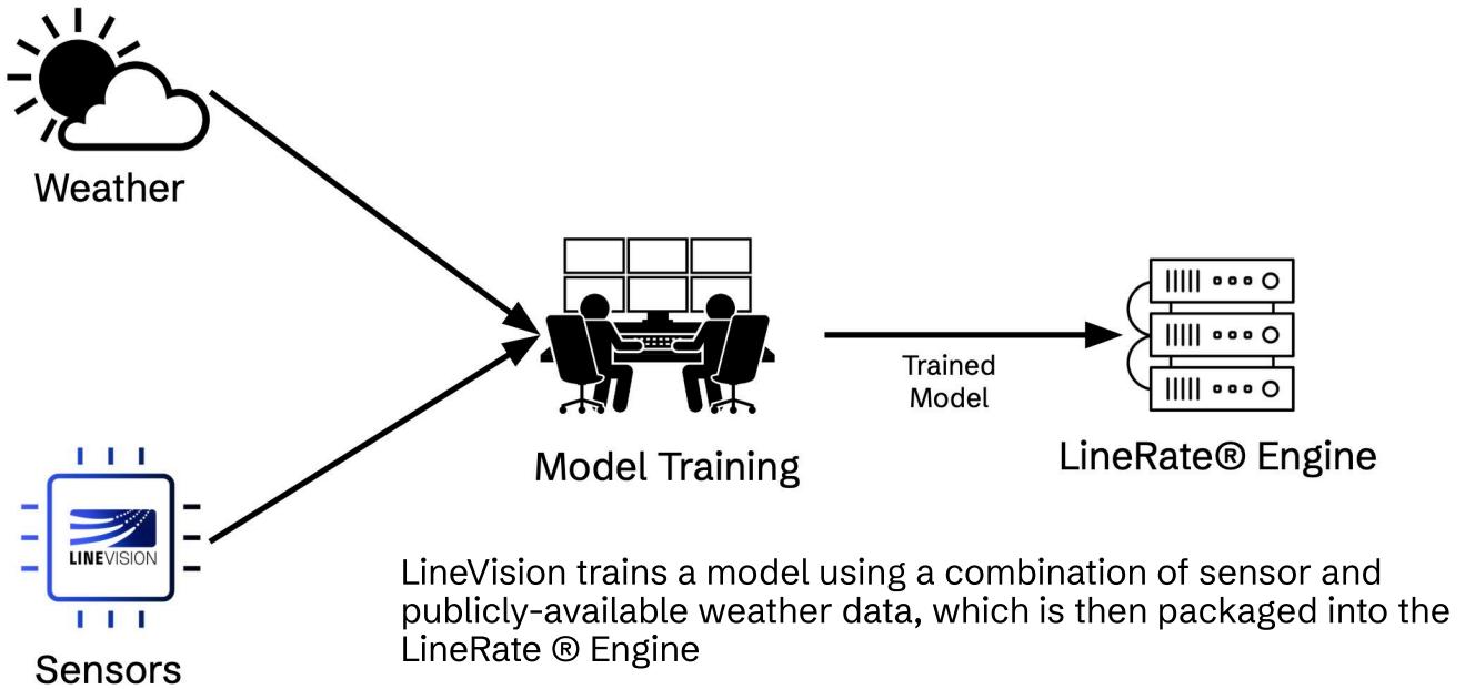
All logic and intelligence are under the Transmission Owner's control and are deployed in adherence to their own security and compliance standards. Aside from wind speed and wind direction, which can be independently verified for accuracy, the LineRate Engine is packaged with all the information it needs to calculate DLR and any other advanced ratings.
