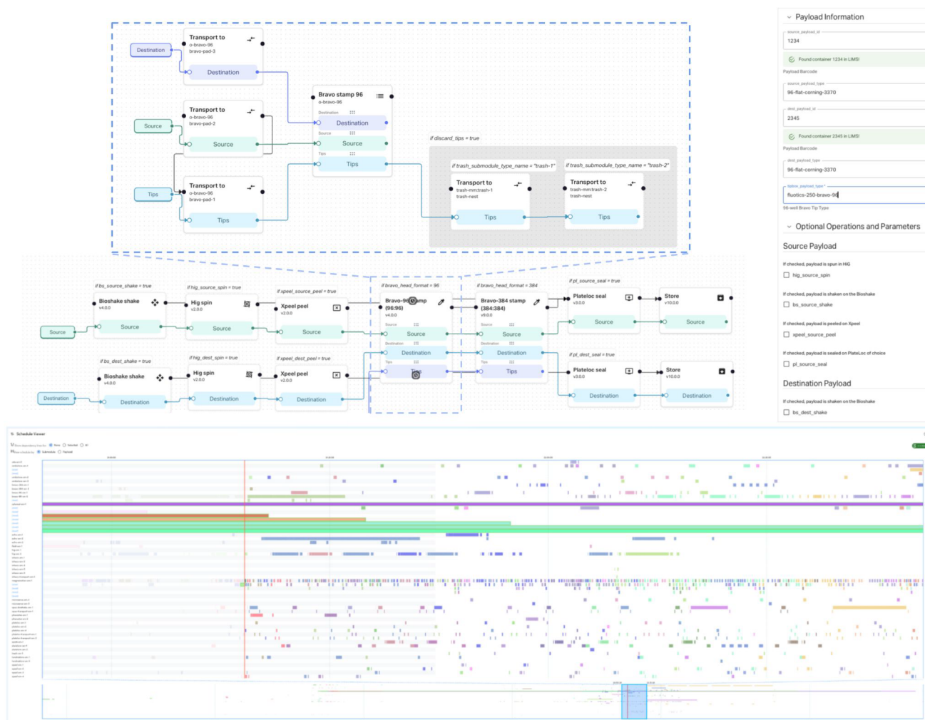
Figure 6: Ginkgo's Catalyst Software lets users build, launch, and monitor complex protocols. Protocols are built from operations (middle), which are composed of lower-level recipes (top) providing control at all levels of abstraction from individual devices to system. Launch forms collect payload and parameter information to customize each run. In-progress and scheduled runs are monitored with a real-time web-based UI (bottom) with each line representing a distinct protocol and the colored bars representing time on distinct devices.
