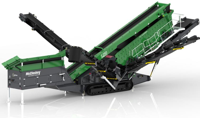
The S250 features 900mm (36") wide side conveyors and 800mm (32") wide auxiliary conveyors for higher material flow. All conveyors have individual speed adjustment giving superior material flow control. The Reversible Cross Conveyor removes unwanted chutes which stops blockages and reduces maintenance required. The operator is able to change from a 3-way split to a 4-way split by turning a lever.
