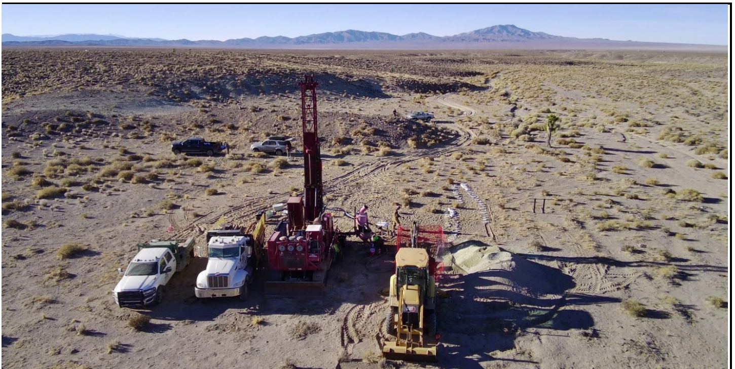
TRACK MOUNTED RC DRILL RIG ON SITE AT ALKALI FLATS
