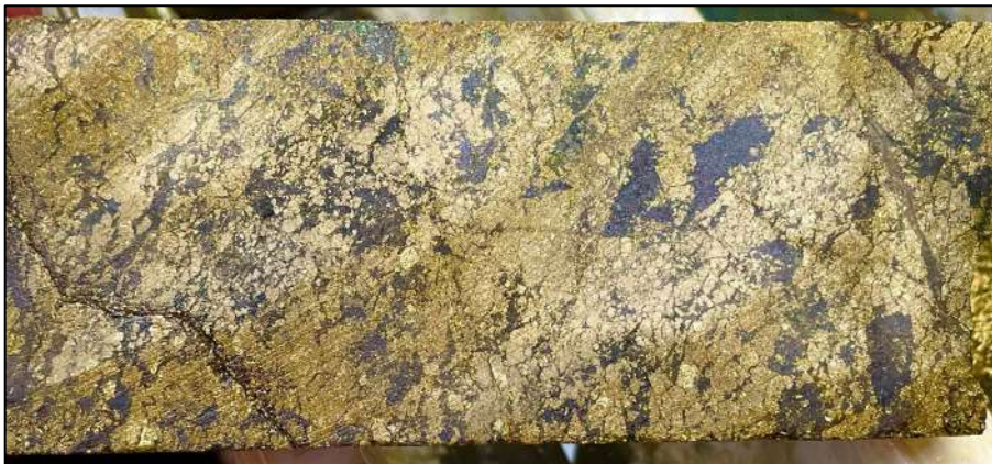
Photo of drill core from SDD005 (353.5m), showing high-grade IOCG style pyrite-chalcopyrite-bornite magnetite mineralization (353-354m: 1.3% Cu, 0.49g/t Au).
