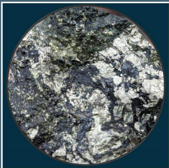
KH21-43 @ 479m: Quartz-carb-mag-sulphide (py-cpy) vein Mineralization
