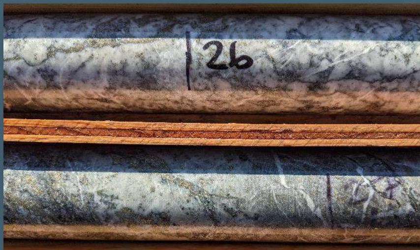
KH21-45 @ 26m: Gold-bearing Quartz-carb-sulphide veins
