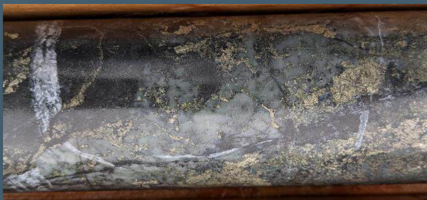
KH21-44 @ 371m: Quartz-Magnetite-Sulphide (py-cpy) vein Breccia
